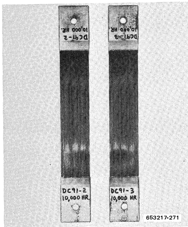
Figure 12-71 G/PI Long-Term Specimens After 10,000 hr of Flight Simulation Exposure
