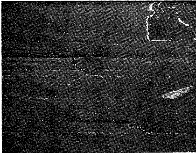
Figure 12-32 Enlarged View of Surface Cracks Found in Heated Zones of B/Al Crossply Specimens After 200 hr of Simulation Exposure at 505 K (450° F), Specimen EC82-3
