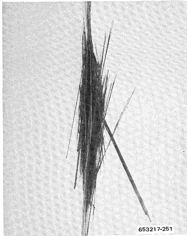
Figure 12-51 Edge View of G/E Long-Term Specimen BC91-4 Showing Exposed and Broken Graphite Filaments and Extensive Delamination. (Specimen was removed from test after 4524-hr)
