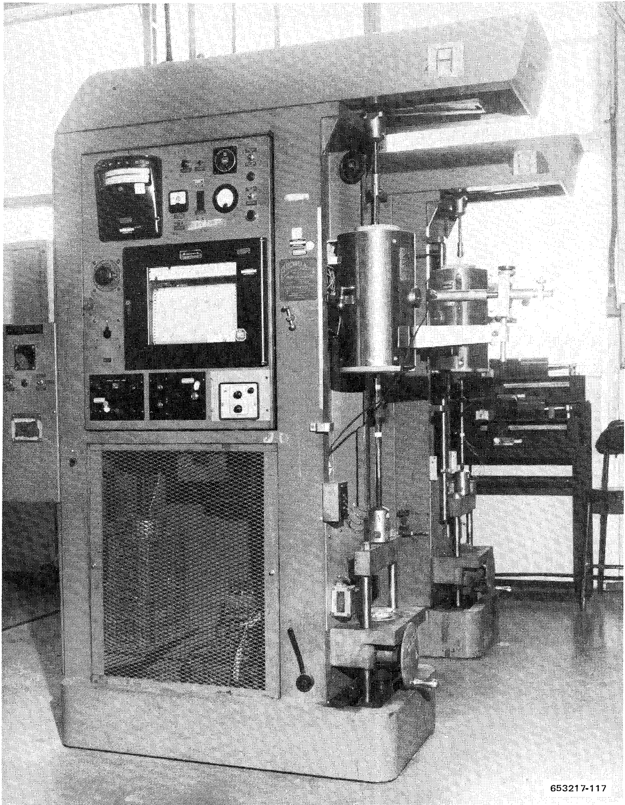
Figure 10-2 Creep Testing Apparatus
