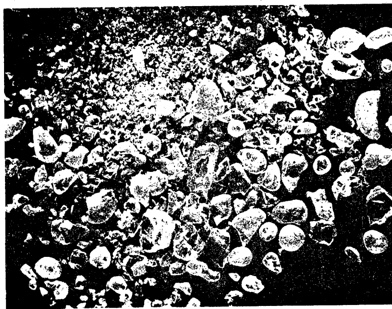
Figure 5A.—Photographs of Polymer Fragments Dislodged from Concrete Voids (Top) MMA-TMPTMA fragments from nonexposed specimen. Photo P801-D-77364 (Bottom) MMA-TMPTMA fragments from 250° F vapor specimen exposure. These fragments show no obvious alteration from exposure. Photo P801-D-77365
