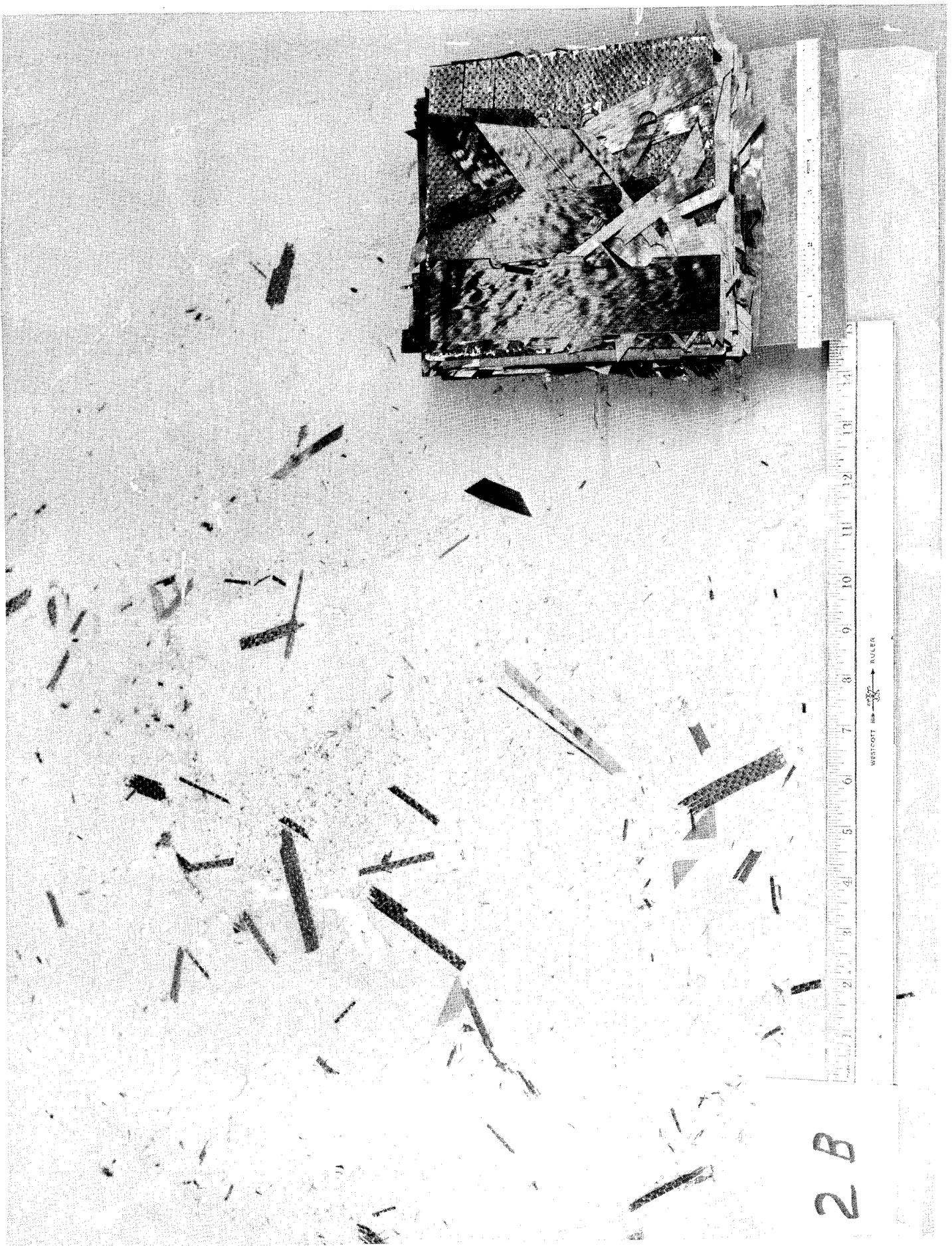
Figure 61 Hybrid System #2b After Burn, Impact, and Air Flow Test
