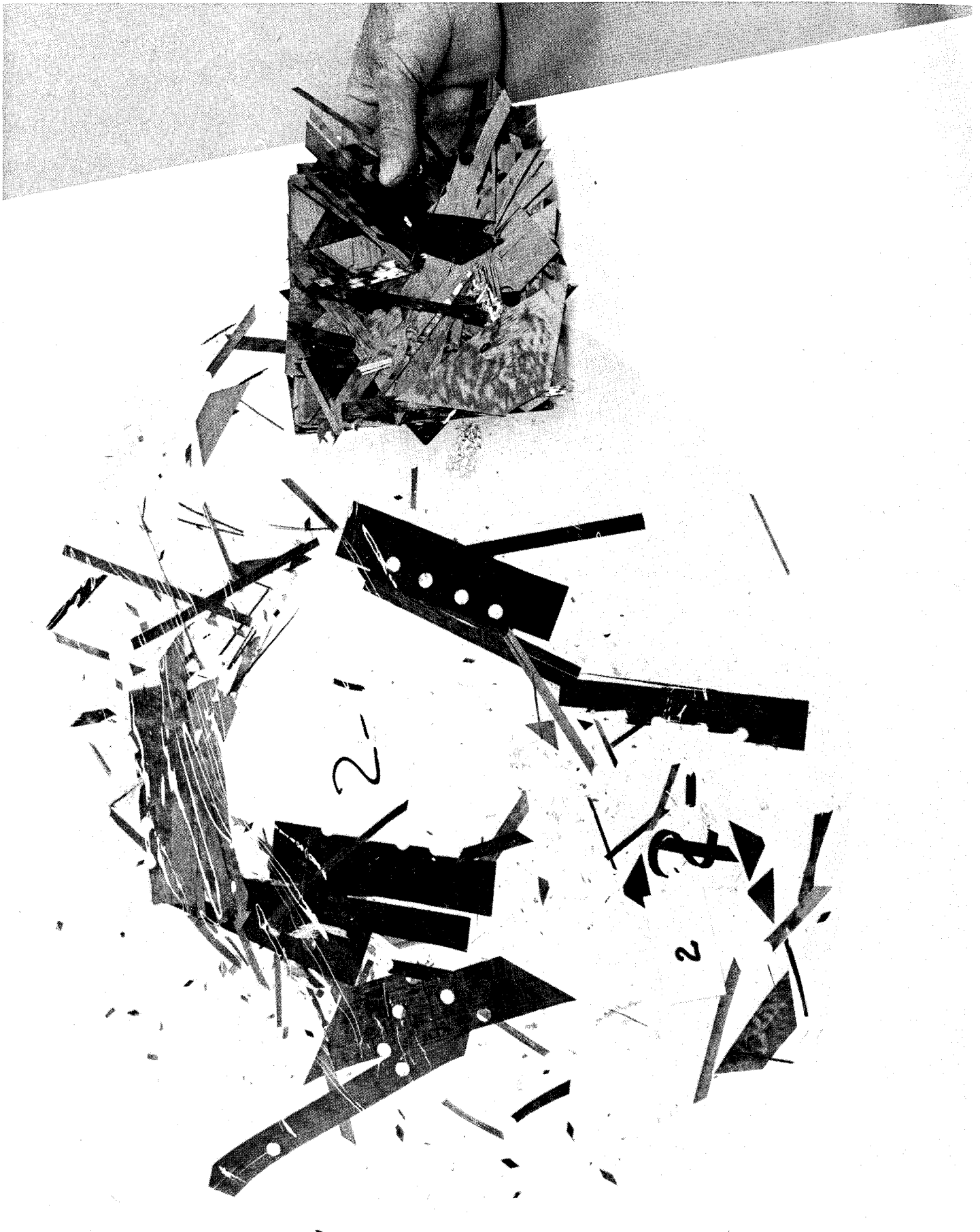
Figure 59 Baseline System #2 After Burn, Impact, and Air Flow Test
