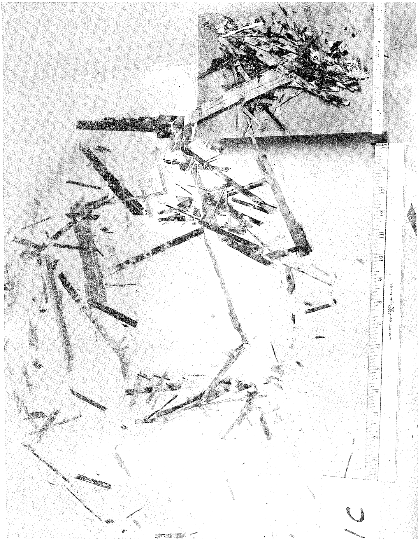
Figure 57 Hybrid System #1c After Burn, Impact, and Air Flow Test
