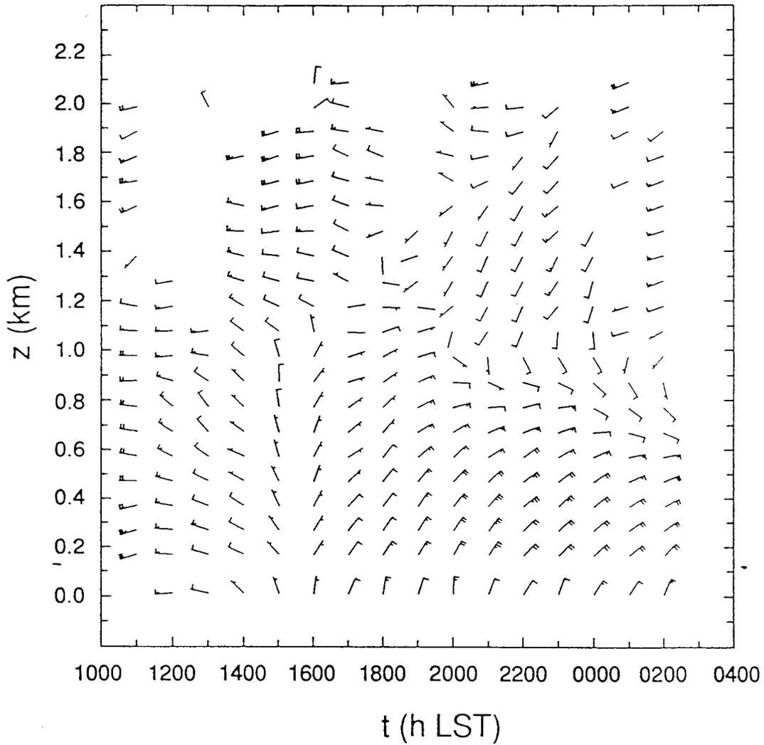
Figure 1b. Hourly averaged winds measured by the Seneca boundary layer profiler and collocated PAM 41, from 1100 LST on 20 February to 0200 LST on 21 February. Each half barb represents 5 knots ( $\approx 2.5$  m/s) and each full barb represents 10 knots ( $\approx 5$  m/s). The passage of the deformation flow is seen in the wind shift between 1400 and 1700 LST.
