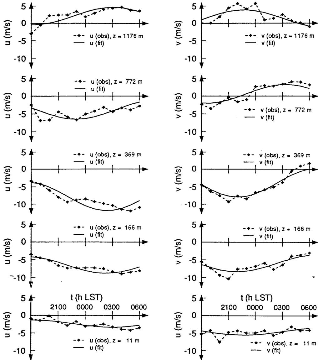
Figure 3b. Plots of observed and least-squares fit  $u$  (left) and  $v$  (right) versus time. From bottom to top: surface PAM station, lowest level of Seneca boundary layer profiler, level of jet maximum and largest-amplitude inertial oscillation, an intermediate upper level, and highest profiler level used.
