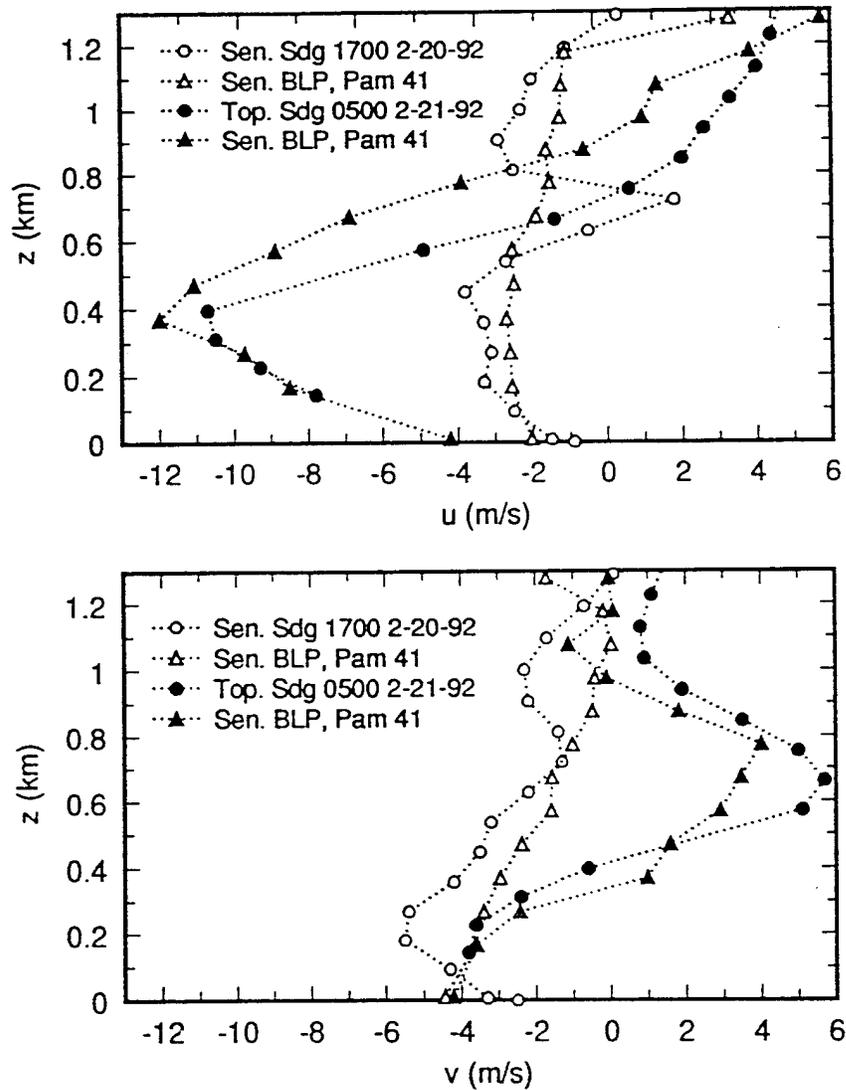
Figure 3a. Comparison of vertical profiles of zonal wind  $u$  (upper) and meridional wind  $v$  (lower) taken by the Seneca boundary layer profiler and nearest available soundings (Seneca CLASS sounding and Topeka NWS sounding). The two times, 1700 LST on 20 February and 0500 LST on 21 February, are near the beginning and near the end, respectively, of the period of inertial oscillation being discussed.
