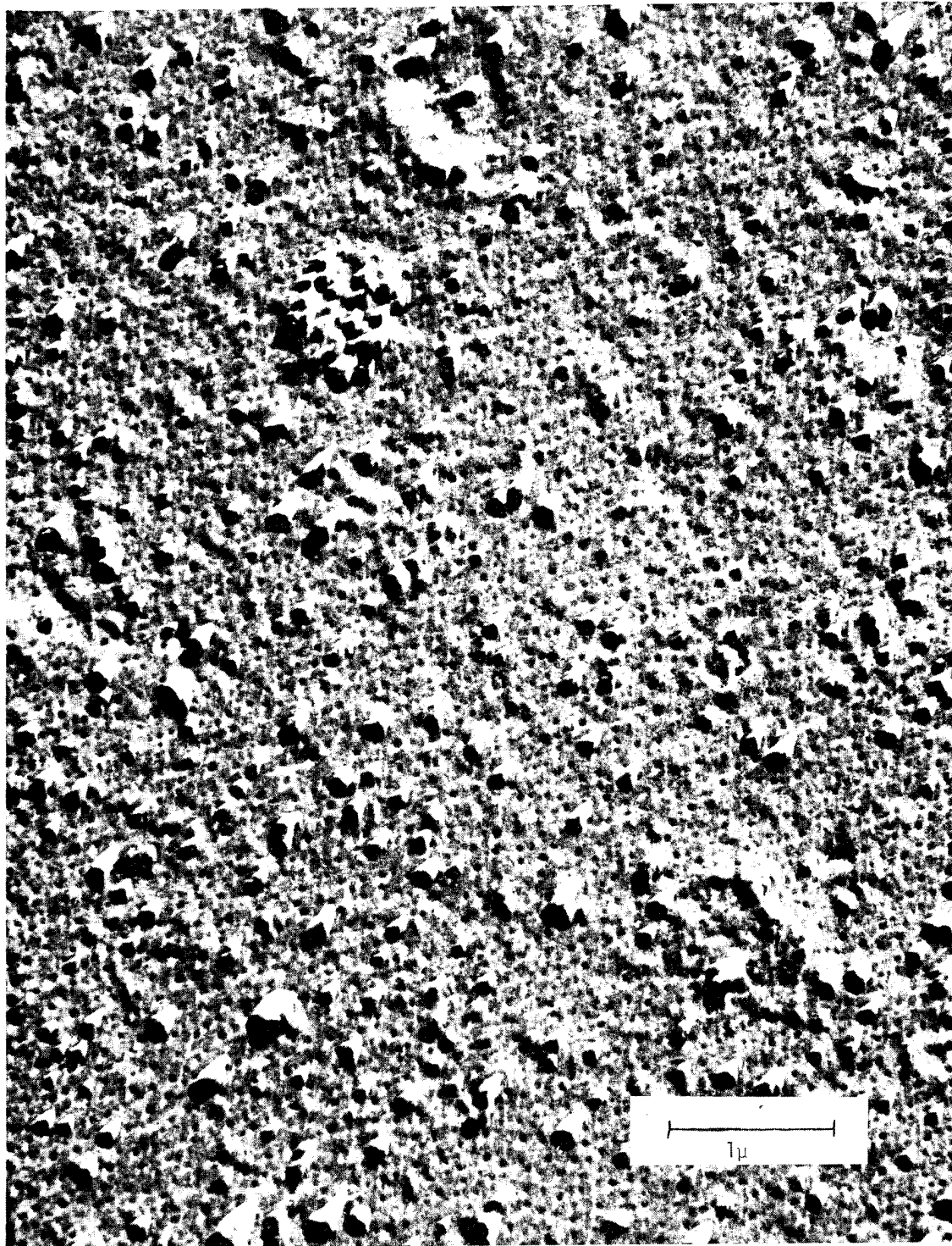
FIGURE 43. ELECTRON MICROGRAPH OF SPECIMEN S-8441-11-4: RESIN S-263 + 7.5 pph HYCAR CTBN. 30,500X.
