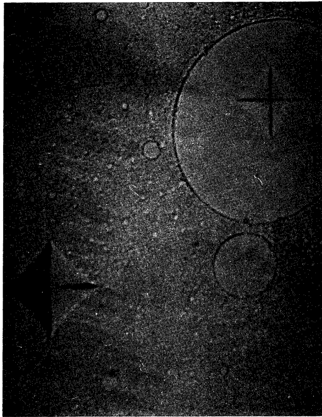
FIGURE 39. VICKERS MICROHARDNESS INDENTATIONS SHOWING THE DIFFERENCE IN MARKINGS BETWEEN THE PARTICLES AND THE MATRIX. POLARIZED LIGHT. 500X.
