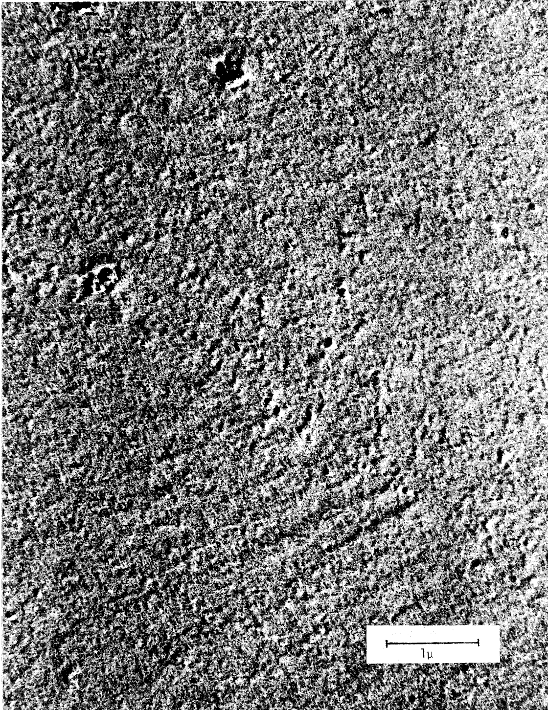
FIGURE 42. ELECTRON MICROGRAPH OF SPECIMEN S-8441-11-3: RESIN S-263 + 5 pph HYCAR CTBN. NOTE THE PRESENCE OF THE FEW DISPERSED PARTICLES. 30,500X.
