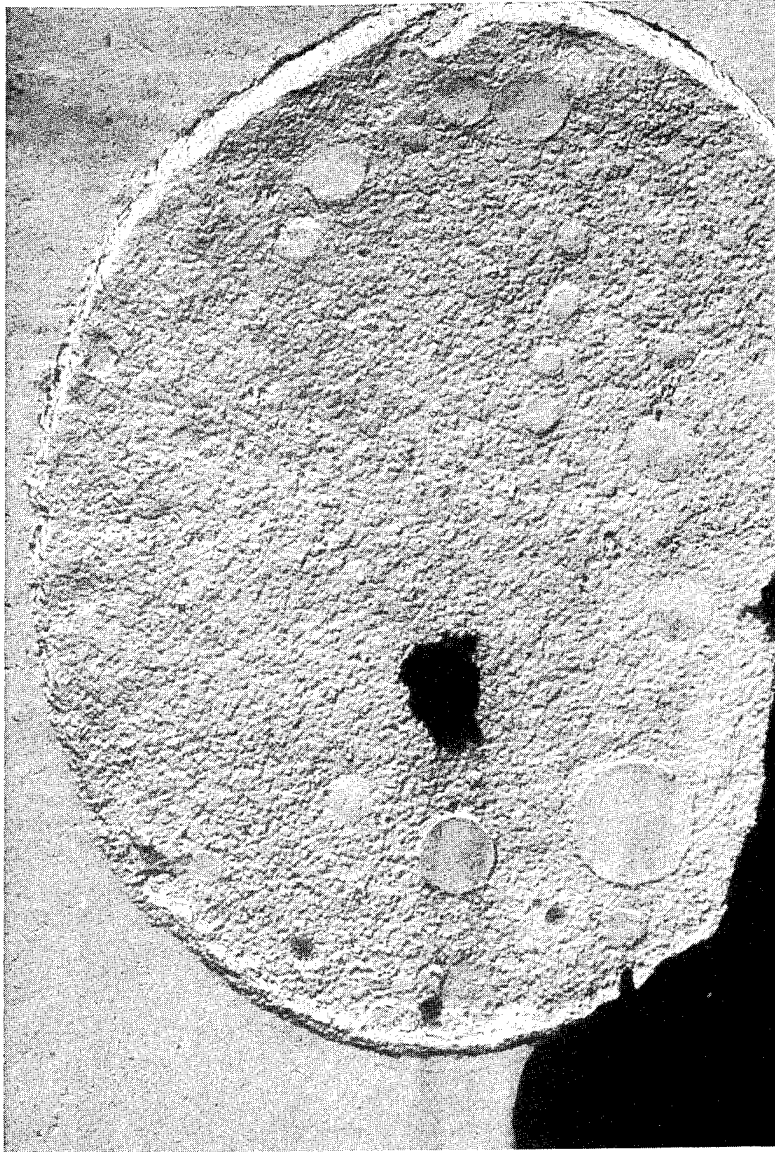
FIGURE 33. ELECTRON MICROGRAPH OF SPECIMEN S-8337-100-6: LAMINAC 4173 ALKYD/STYRENE/HYCAR CTBN (42/ 53/5). 7,200X.
