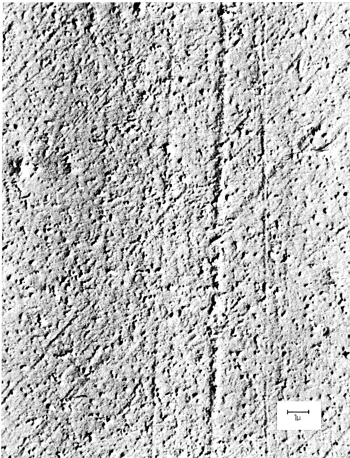
FIGURE 44. ELECTRON MICROGRAPH OF SPECIMEN S-8441-11-5: RESIN S-263 + 10 pph HYCAR CTBN. 11,000X.
