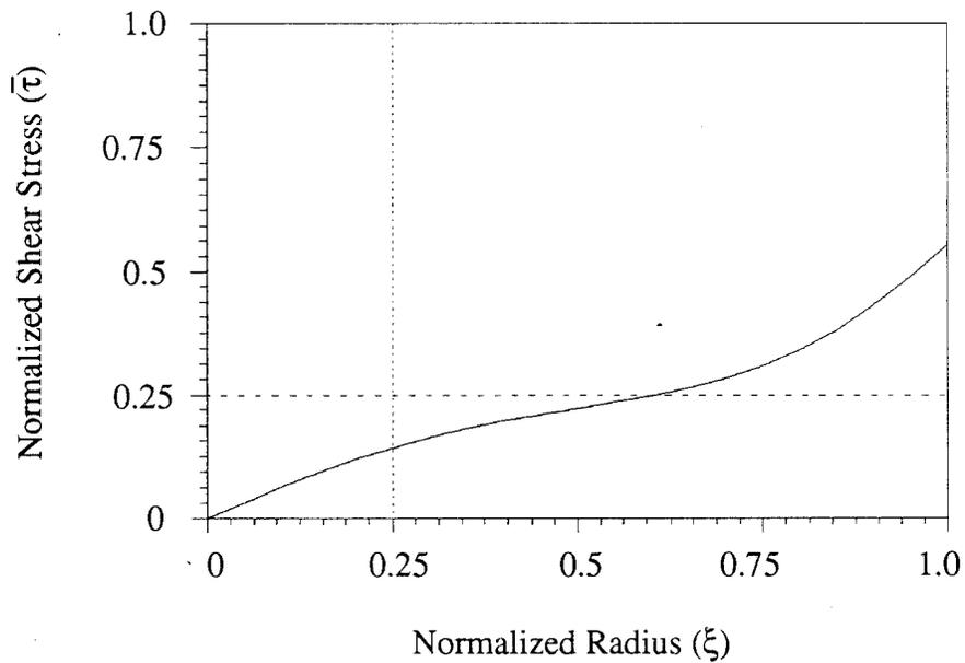
Figure 5. Shear Stress Profile as a Function of Radial Location at 0.025 Nondimensional Time
