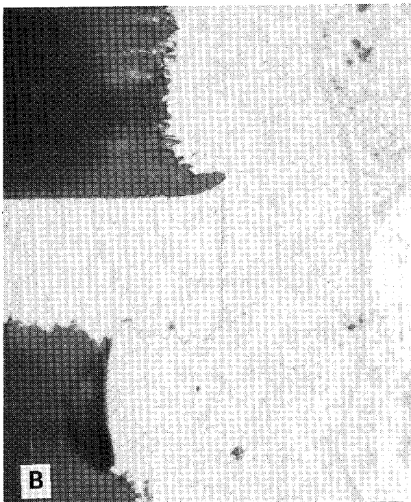
B. ETCHBACK EFFECTIVE ON ONE SIDE. ETCHED, 400X.
