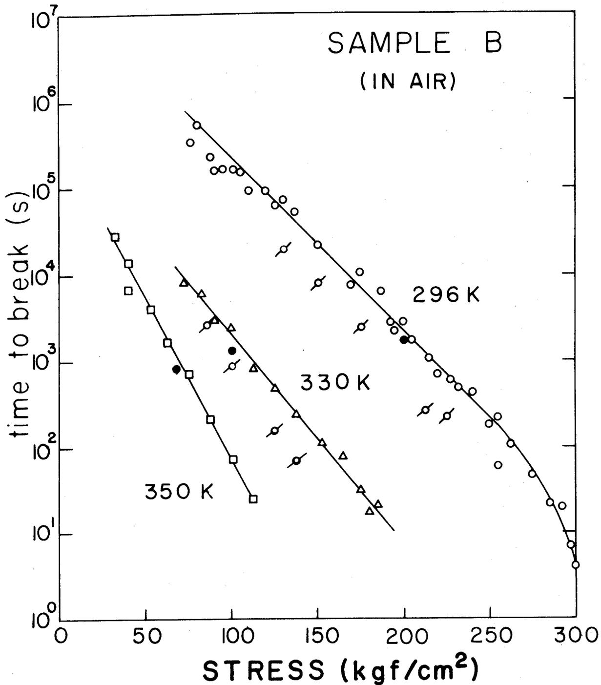
7.2 Log. Time-to-Break Versus Static Load for Polyethylene Sample B ( $M_w = 90,000$ ). Open Symbols - in air,  $\circ$  - presoaked in motor oil at 60°C for 24 hours,  $\square$  - presoaked in hexane at 23°C for 24 hours.
