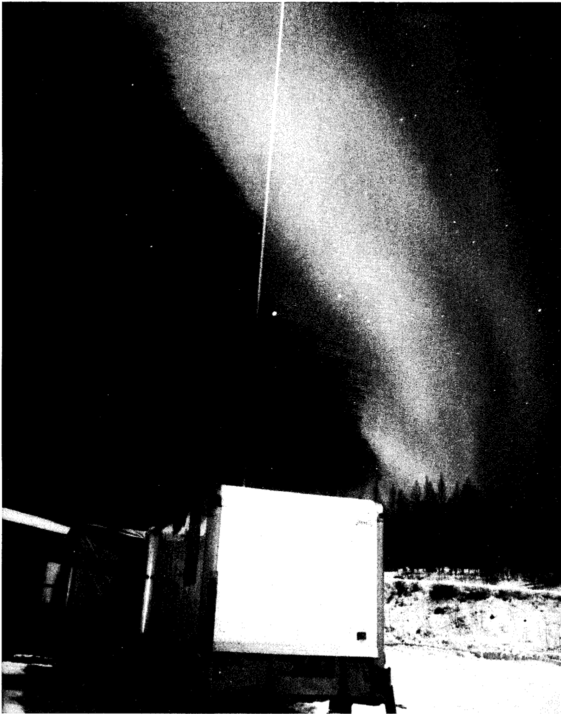
The Geophysics Laboratory made LIDAR measurements in Alaska in 1986. The campaign measured atmospheric density in support of Air Force vehicles making a high-latitude reentry. In the background, the northern lights move across the sky.
