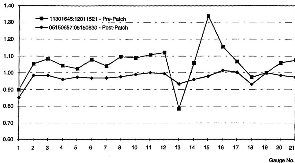
Figure 2. Normalised RMS Strain Ratios without Patch Influence
