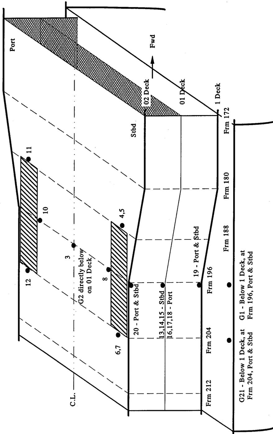
Figure 1: Strain Gauge Locations - HMAS SYDNEY.
