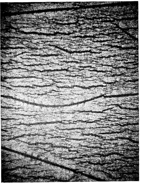
FIGURE 1: Cracks and fissures in polypropylene after 15-min. etch in hot chromic-sulfuric acid solution. (75X, dark field)
