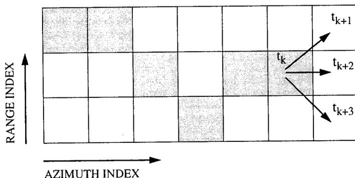
Figure 3.10: The tracking of discrepant tiles. The shaded tiles form a track that has been extended up to a tile  $t_k$ . The track is further extended if one of the tiles,  $t_{k+1}$ ,  $t_{k+2}$ , and  $t_{k+3}$ , is discrepant.
