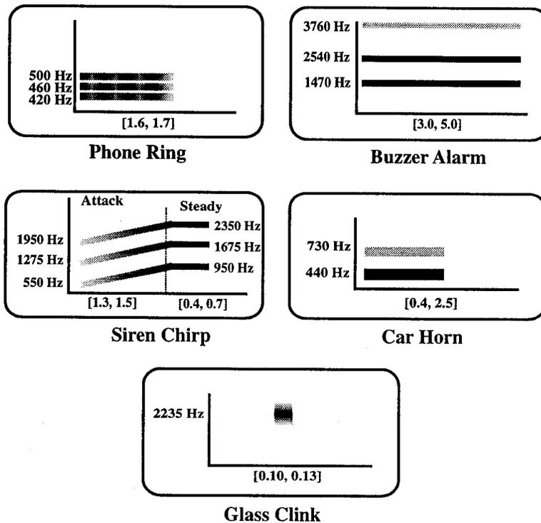
Figure B.7.13: *IPUS Source Database*. The vertical axis represents frequency and the horizontal axis represents time in seconds. The energy changes for each microstream are represented qualitatively by the shading gradations. Note that *Phone-Ring* is a ring from a phone different from the one in Figure B.2.3.
