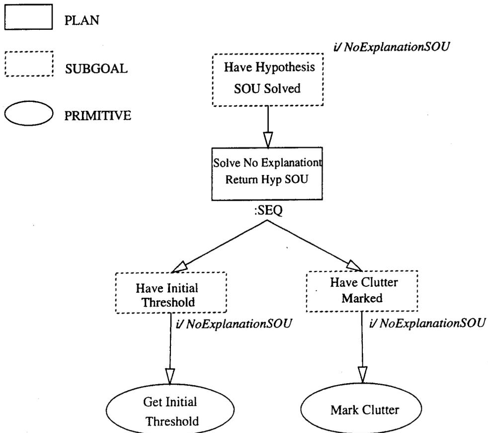
Figure 3.14: A pictorial representation of control plan strategy for pursuing a subgoal, `HaveHypothesisSOUSolved` with input `NoExplanationSOU` attached to a *return* hypothesis.
