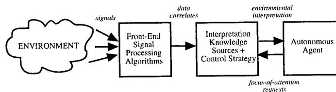
Figure B.1.1: *Classic Knowledge-Based Signal Processing Architecture.* This paradigm imposes a unidirectional control flow that limits interpretation processes' analysis to only the single set of observations afforded by the fixed signal processing. Interpretation processes do not usually provide structured feedback to the front-end about either the adequacy of the signal processing outputs to be interpreted or any anticipated signal behavior.
