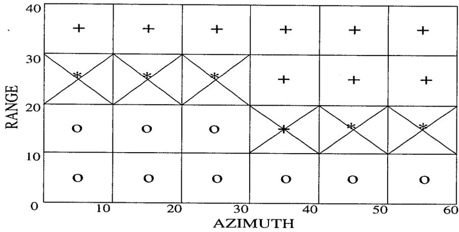
Figure 3.11: Horizontal boundary. The two separate horizontal boundaries are connected by declaring a “+” tile to be discrepant. The tiles included in the boundary are shown with a cross.
