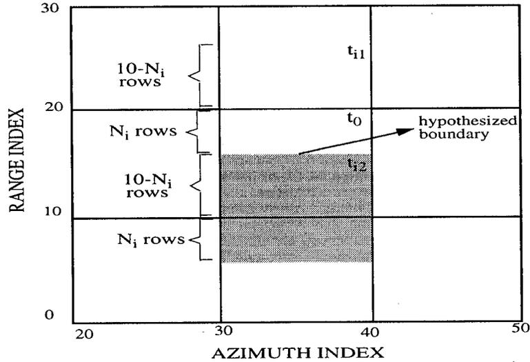
Figure 3.13: The formation of two tiles,  $t_{i1}$  and  $t_{i2}$ , under the hypothesis that the top  $N_i$  rows in a tile,  $t_0$ , belong to the subregion located above the tile.
