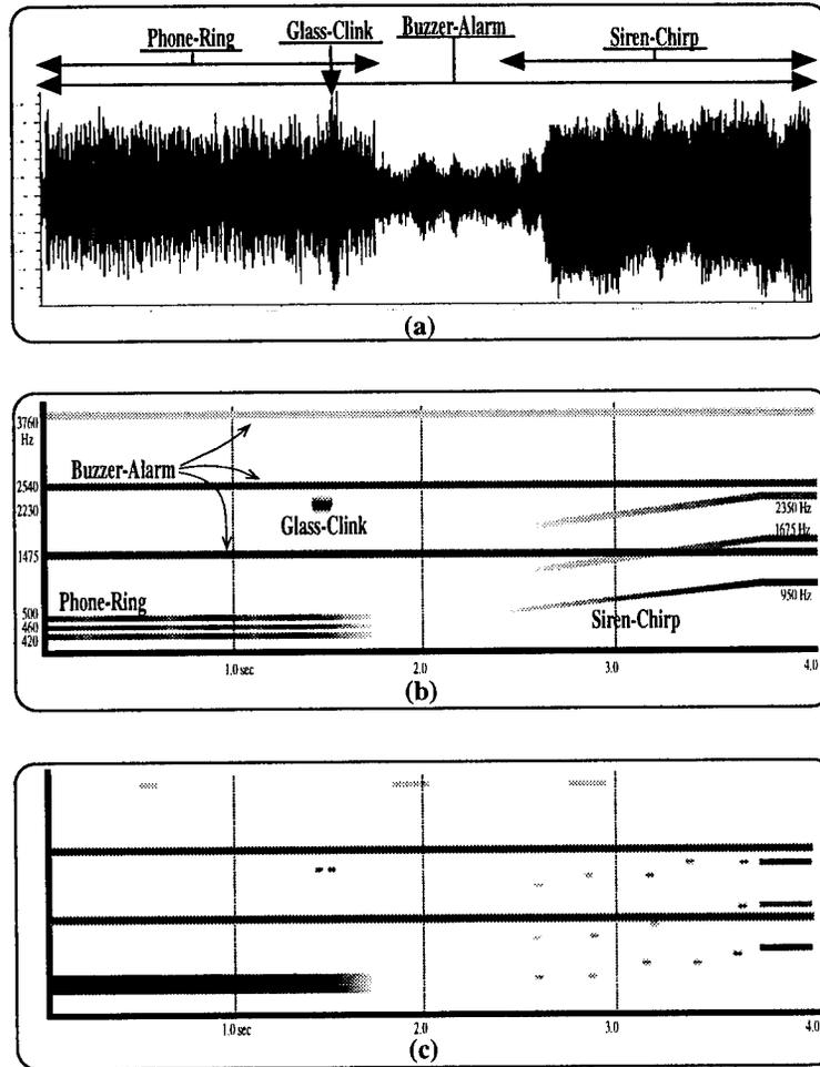
Figure B.7.12: *Acoustic Scenario Events*. Figure B.7.12a shows the scenario's time-domain waveform. Figures B.7.12b and B.7.12c show the scenario's frequency-domain events. Darker shading indicates higher frequency-domain energy.
