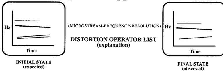
Figure B.6.6: *Microstream Frequency Resolution Operator from the Acoustic Interpretation Testbed. When applied to a state, the operator replaces each set of expected microstreams whose members are closer than  $SAMPLE-RATE/WINDOW-LENGTH$  with a single microstream, reflecting the resolving limits associated with the current value of  $WINDOW-LENGTH$ . In the short example illustrated, this operator effectively reduces the differences between the expected state and the observed state.*
