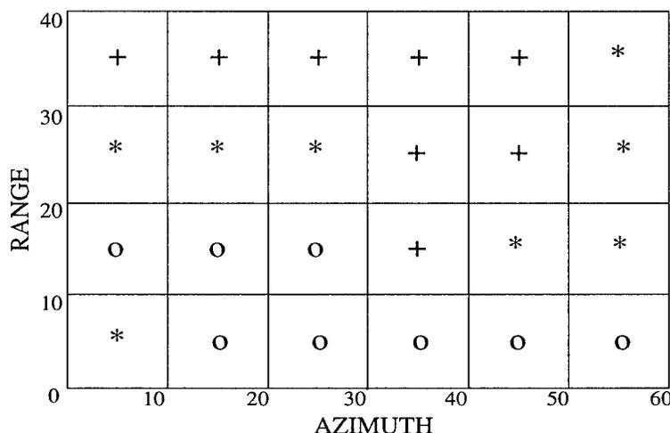
Figure 3.9: The groups of tiles in the range-azimuth plane. The two homogeneous subregions,  $W$  and  $L$ , are labeled by “+” and “o”, respectively. The discrepant tiles are indicated by the symbol “\*”.
