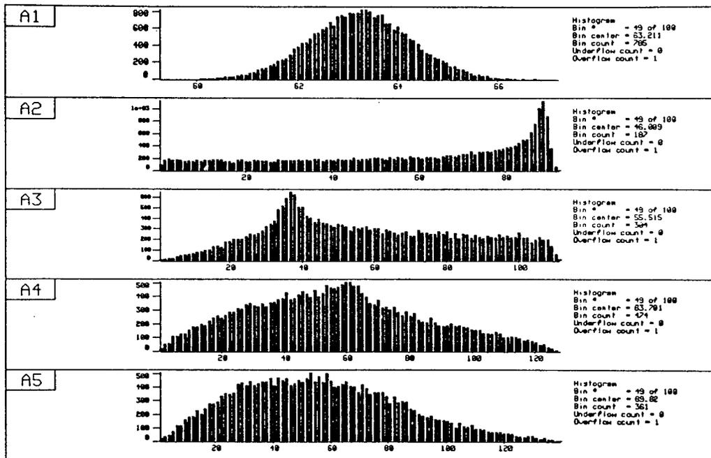
Figure 4.4.1: Amplitude pdf of the sum of  $N_J$  equal amplitude jammers – A1)  $N_J = 1$ ; A2)  $N_J = 2$ ; A3)  $N_J = 3$ ; A4)  $N_J = 4$ ; A5)  $N_J = 5$ .
