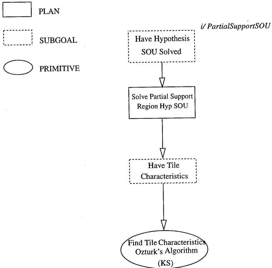
Figure 3.16: A pictorial representation of the plan, HaveHypothesisSOUSolved with input PartialSupportSOU attached to a *region* hypothesis.
