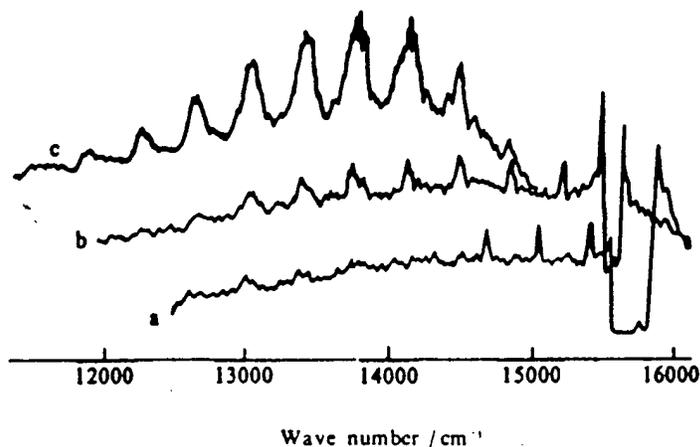
Figure 4.  $\text{CuCl}_2$  LIF spectra and red fluorescence Fourier transform (FT) spectrum. Lines a and b represent  $\text{CuCl}_2$  LIF spectra for pumping laser wavelengths at 635nm and 643nm, respectively. Line c represents the red fluorescence FT spectrum.
