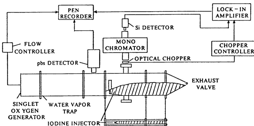
Figure 1. Experimental COIL apparatus. The hatched portion represents the location where the red emission was observed.<sup>2</sup>
