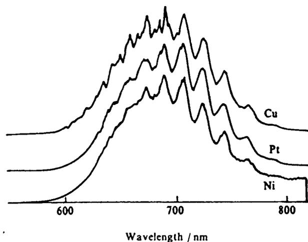
Figure 2. Red fluorescence spectra from different intensifiers
