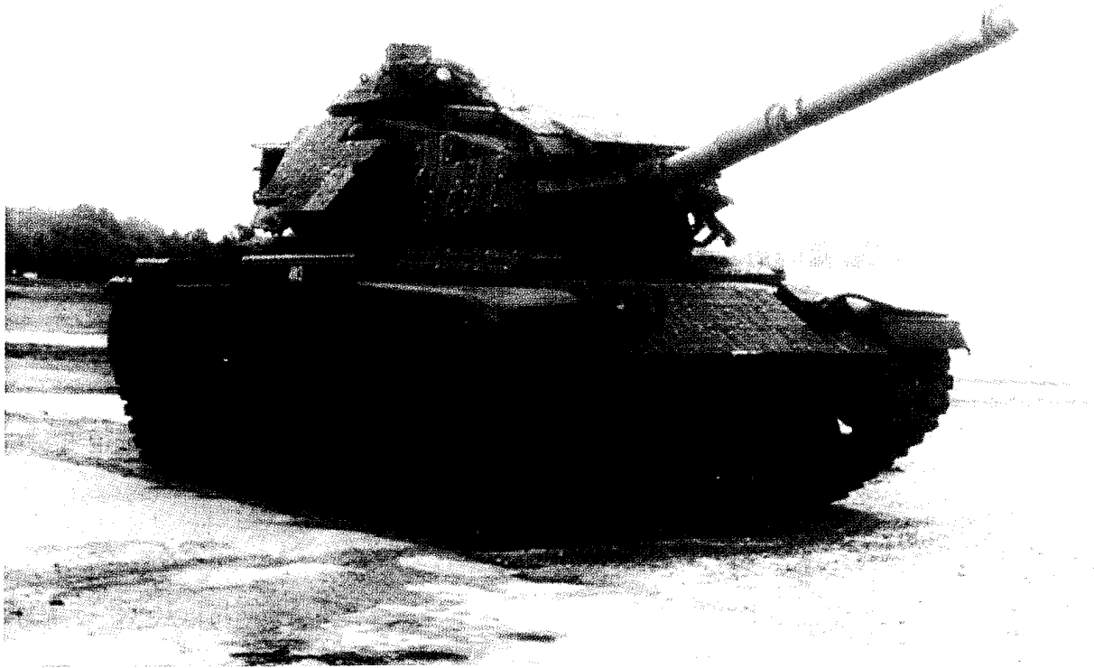
M60A3 Tank With RA Applique—As Used by the Marines in Operation Desert Shield/Storm.
