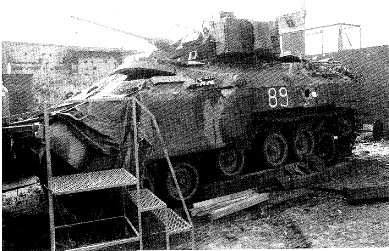
A Firing Against a BFV to Test the Vaporific Effect.
