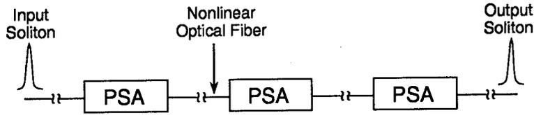
Figure 2: Schematic of a nonlinear optical fiber transmission line in which loss is balanced by a chain of periodically-spaced, phase-sensitive amplifiers (PSA's).
