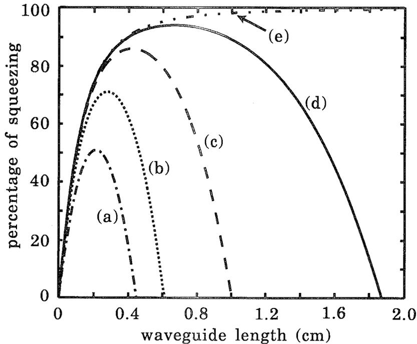
Figure 17: Effect of SSD phase mismatch on squeezing for a Gaussian pump pulse with uniform phase under its pulse profile and without nonlinear absorptio: (a) LO pulse has the same width as the Gaussian pump pulse; (b), (c), and (d) narrow uniform-phase LO pulse, where the LO pulse width is taken to be  $1/2$ ,  $1/4$ , and  $1/8$  of that of the pump pulse, respectively. Curve (e) illustrates the square pump pulse case as a comparison.
