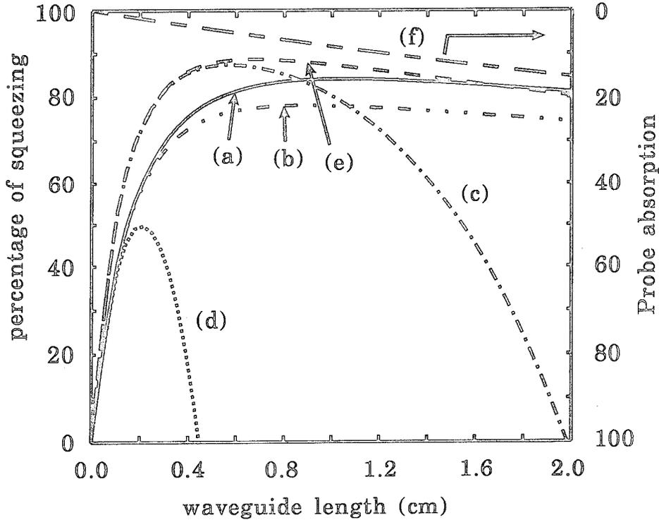
Figure 18: Squeezing with nonlinear absorption: (a) Gaussian pump pulse with nearly matched LO pulse from another waveguide; (b) Gaussian pump pulse with reused pump pulse; (c) Gaussian pump pulse with narrower uniform-phase LO pulse; (d) Gaussian pump pulse with uniform-phase LO having the same width as the pump; (e) Square pump pulse; (f) Relative pump amplitude  $E_p(l)/E_p(0)$ .
