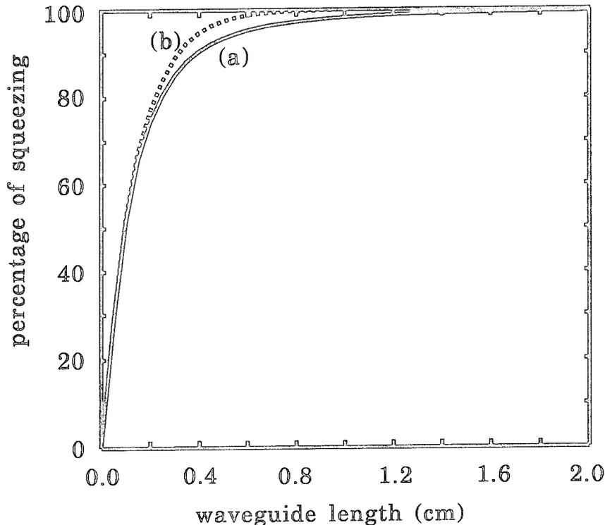
Figure 16: The effect of nonlinear pump-probe phase mismatch  $\Delta\kappa$  on the amount of squeezing, as function of waveguide length for a square pump pulse, uniform phase LO and without nonlinear absorption: (a)  $\Delta\kappa \neq 0$ , and (b)  $\Delta\kappa=0$ .
