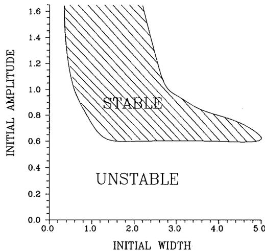
Figure 4: Initial pulse amplitudes  $A$  and widths  $T_0$  which give stable pulse solutions. The initial conditions  $U(T,0) = A \text{sech}(T/T_0)$ , with different values of  $A$  and  $T_0$ , were used. For all initial conditions within the lined region the same final steady-state was reached.
