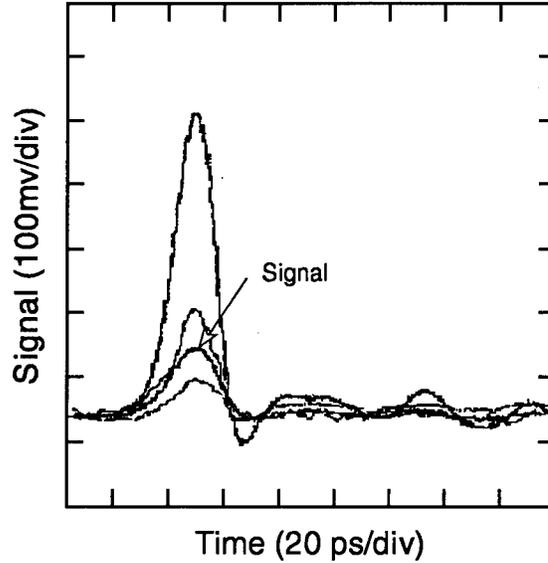
Figure 7: Phase dependence of the signal amplification for  $I_s=40\ \mu\text{W}$  and  $I_p=2\ \text{mW}$ .
