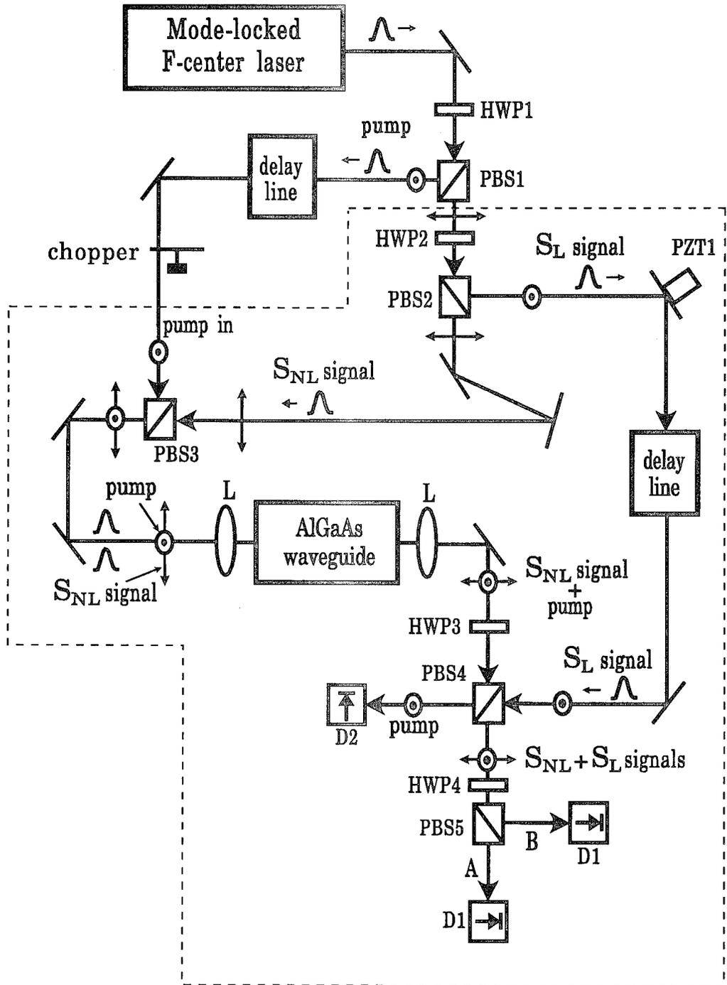
Figure 12: Experimental set up of the Mach-Zehnder configuration for all-optical switching using AlGaAs waveguides.
