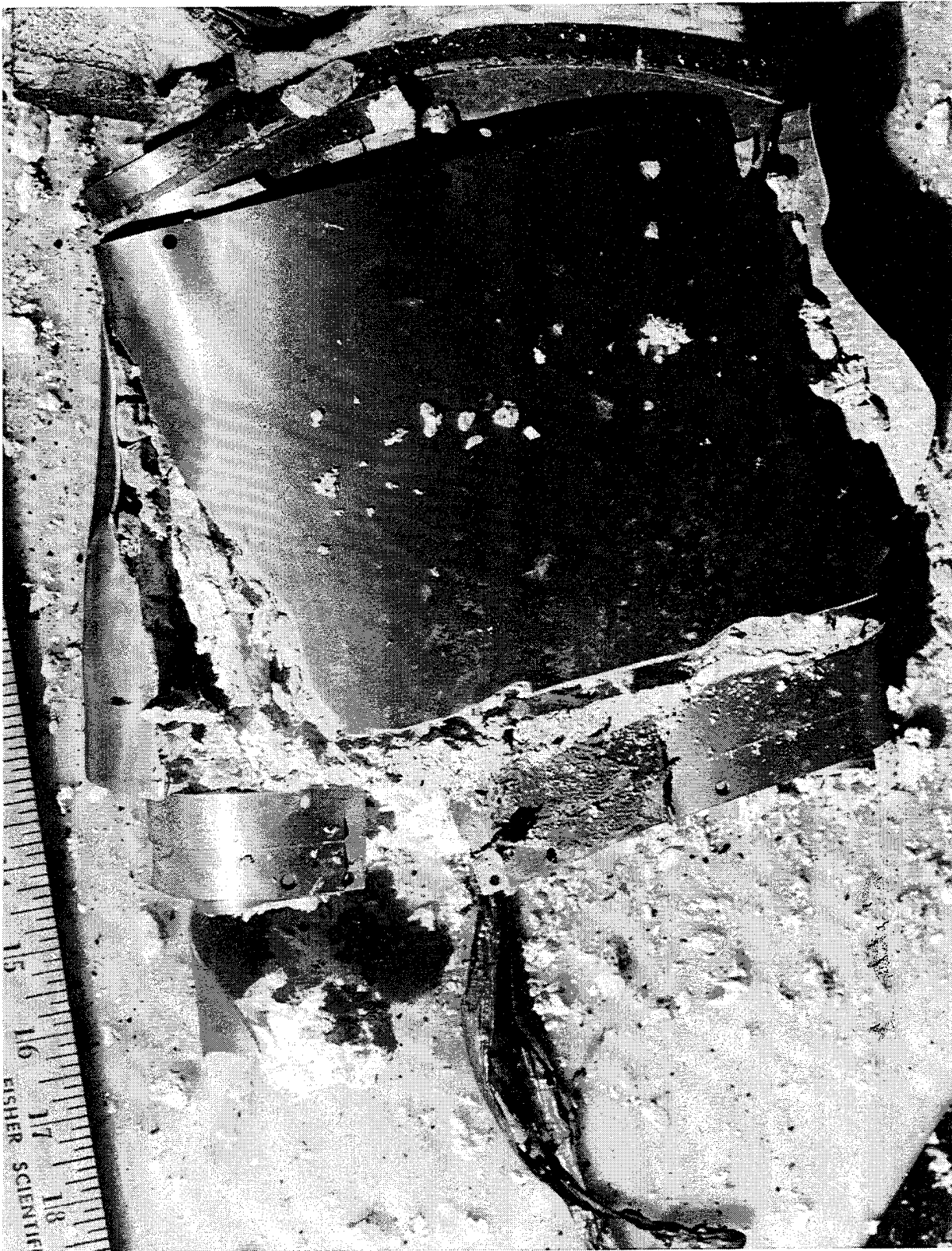
Figure 11. Top view of TOW 2 warhead after being crushed in a no go test.
