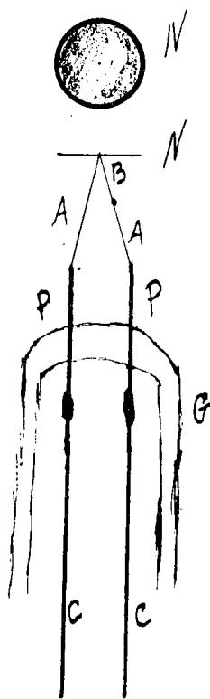
Fig. 1, Diagram of thermoelement device
