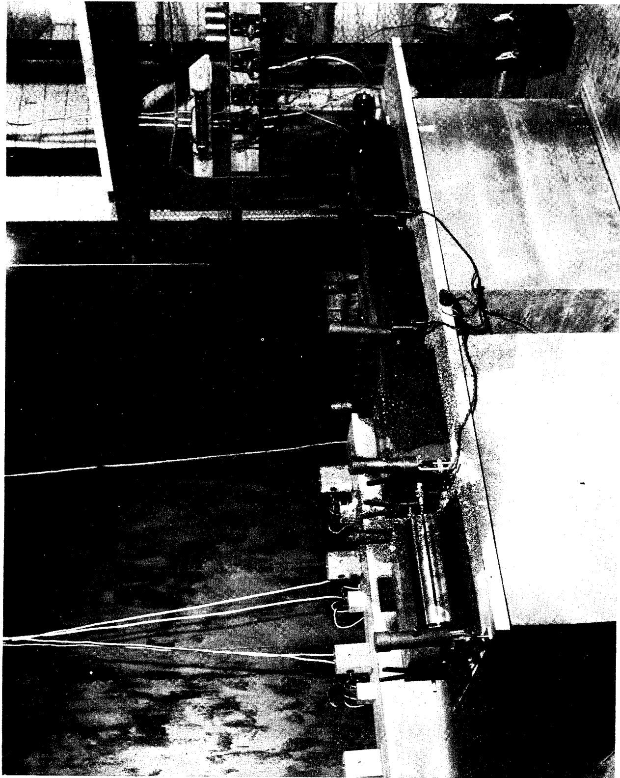
11. General view of the recording room: On the pier in foreground are the recording drums (one uncovered), and the galvanometer lamps; on the pier on left are four of the galvanometers; on the wall are relays for opening and closing the shutters of the instrument on the tower.
