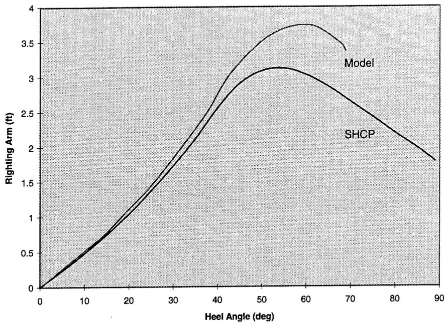
Figure 7. Righting Arm Curve Comparison: Intact Condition
