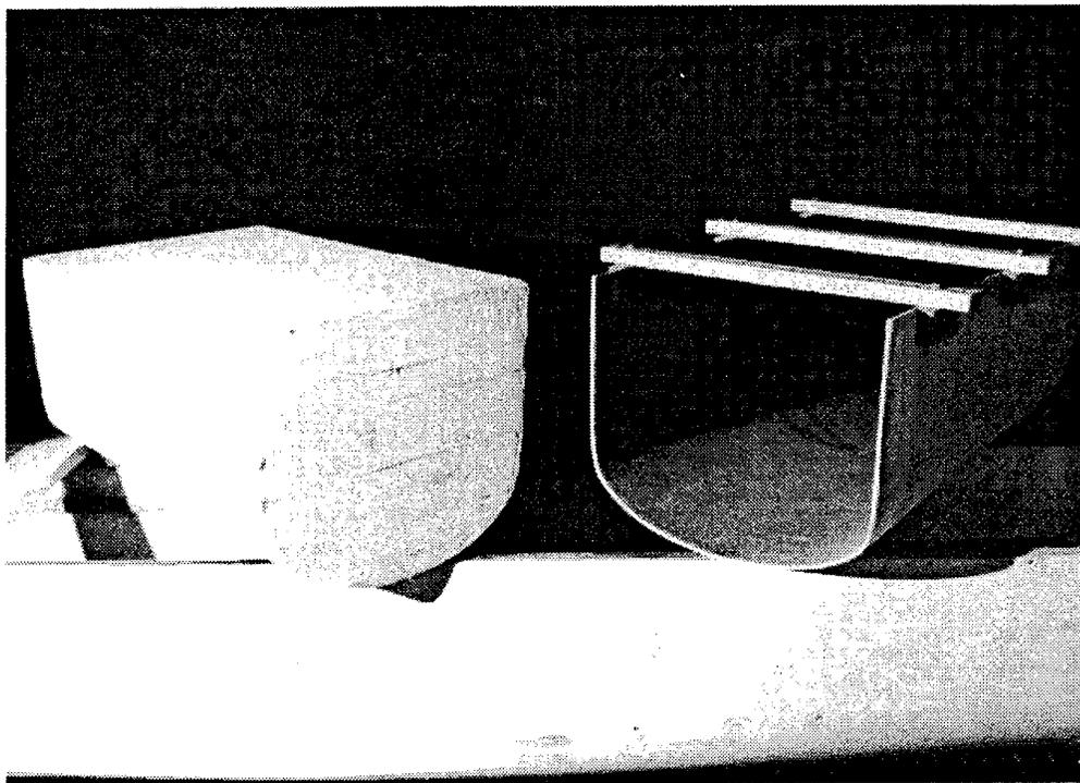
Figure 2. Inner Shell and Inner Foam Inserts
