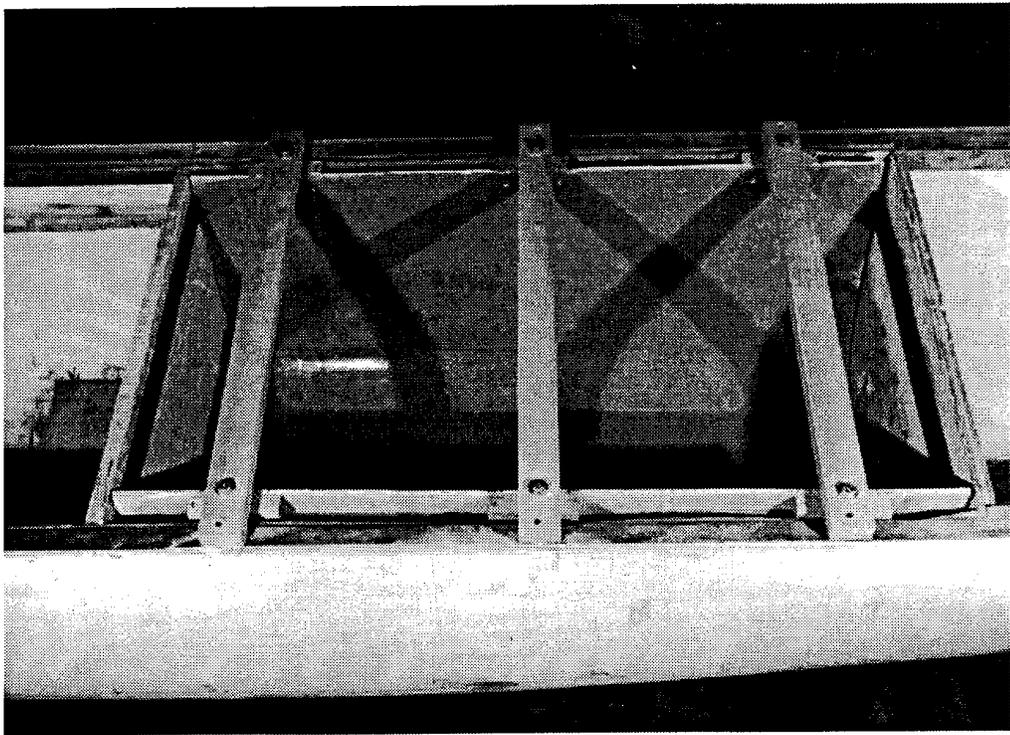
Figure 4. Inner Hull Insert As Placed in Model
