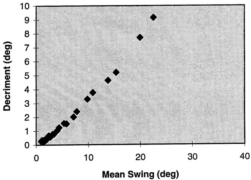
Figure 16. Roll Extinction Data: J-Tank, Outer and Inner Shells Damaged
