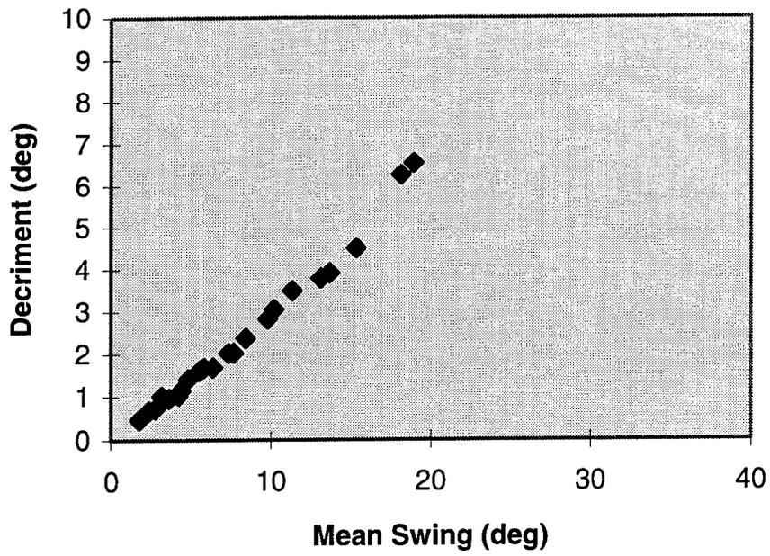
Figure 15. Roll Extinction Data: J-Tank, Outer Shell Damaged
