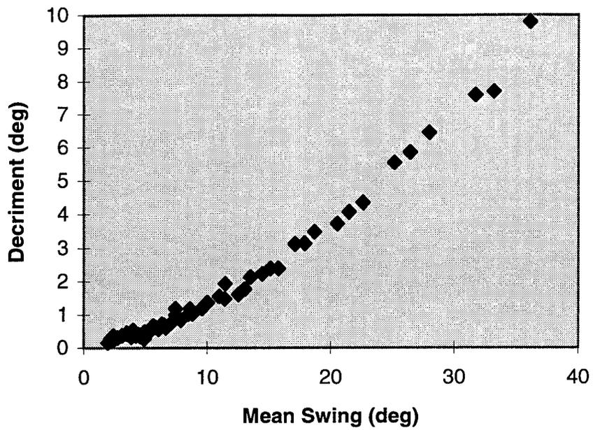
Figure 13. Roll Extinction Data: U-Tank, Outer Shell Damaged
