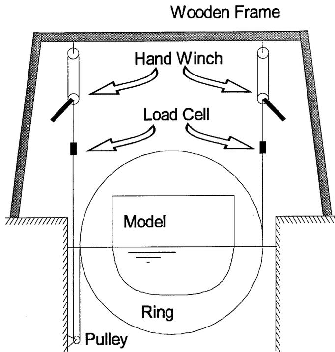
Figure 5. Schematic Diagram of Righting Arm Test Apparatus
