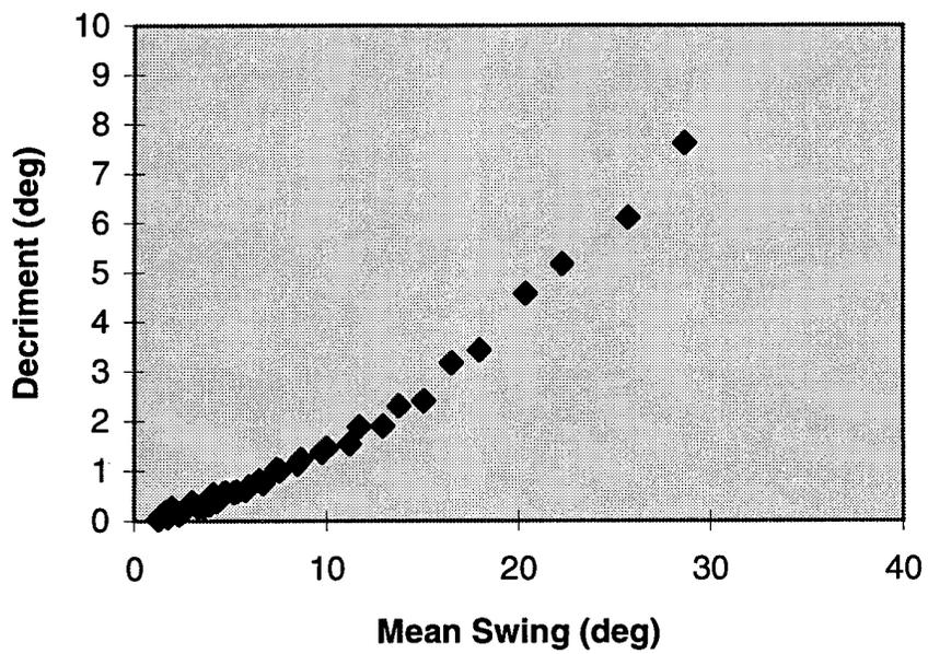
Figure 14. Roll Extinction Data: U-Tank, Outer and Inner Shells Damaged
