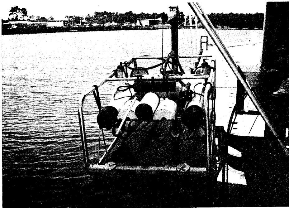
Figure 3. ROV used for potential measurements away from seawall.
