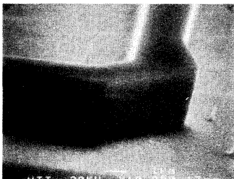
Fig. 6 SEM photograph of the corner mirror. The slightly contrasting layer 1.5 \mu\text{m} under the waveguide top is the InGaAsP core layer.
