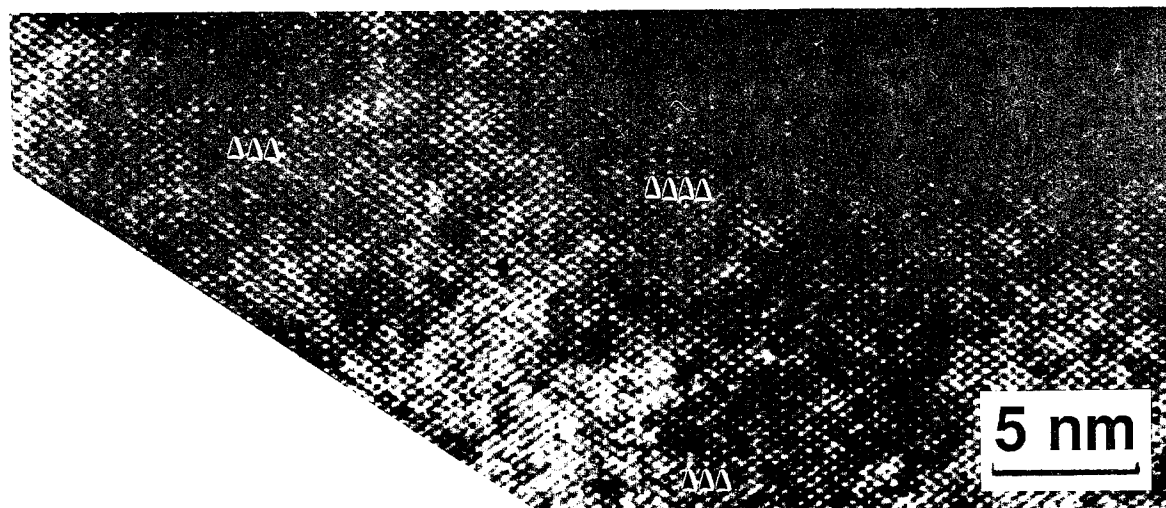
Fig. 4 A (\bar{1}10) cross-sectional high-resolution TEM image of GaAsSb crystal on a (110)InP substrate ( 5^\circ off toward the \langle 00\bar{1} \rangle ) at 500^\circ\text{C} .
