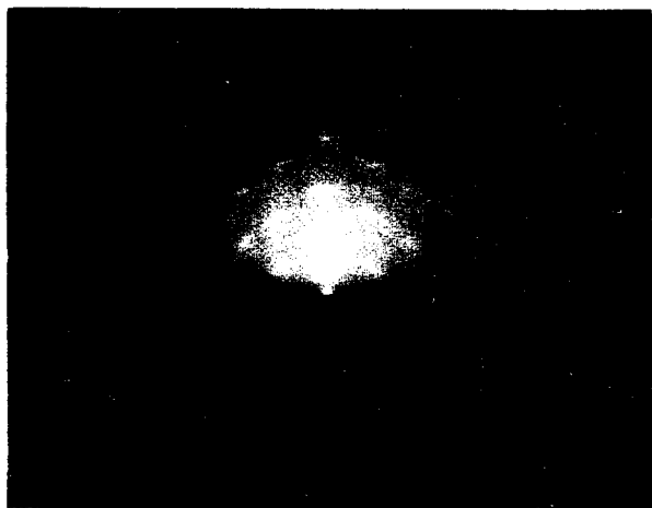
Fig. 3(a). RHEED pattern of InN grown under without-UV irradiation.
