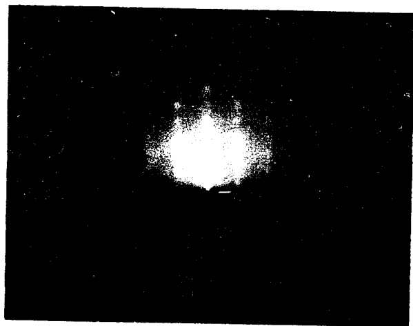
Fig. 3(b). RHEED pattern of InN grown under UV-irradiation.
