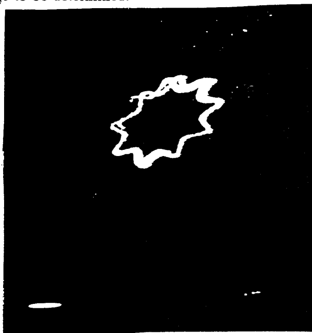
Figure 3. Nine branch star pattern of a 1.0 \mu\text{m} diameter B. subtilis spore particle in the equatorial plane of the ion trap.
