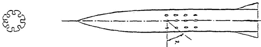
Fig. 4.2 - DIRECT THRUST VECTOR CONTROL USING THRUSTERS
