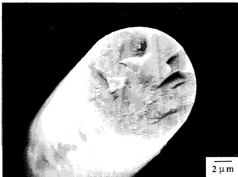
Figure 22(B). Typical Fracture Surface of the Nicalon-Fiber.
