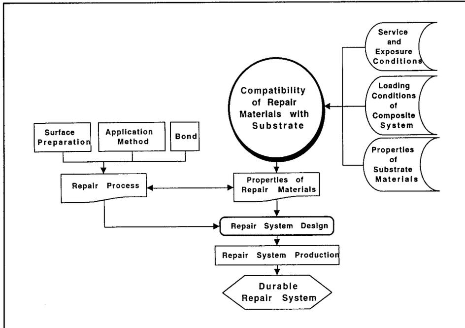
Figure 4. Factors affecting durability of concrete repair system
