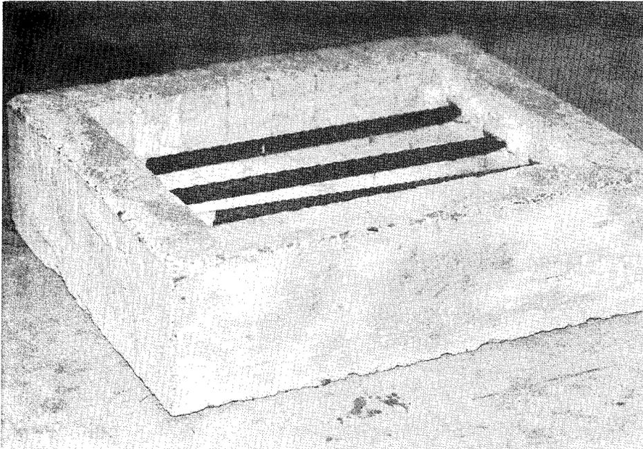
Figure 31. General view of Thoro Shrinkage Test slab
