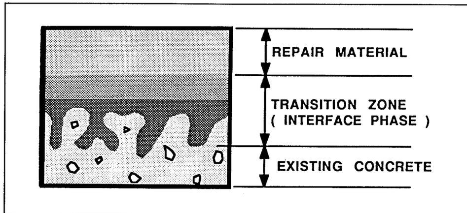
Figure 3. Idealized model of a surface repair system
