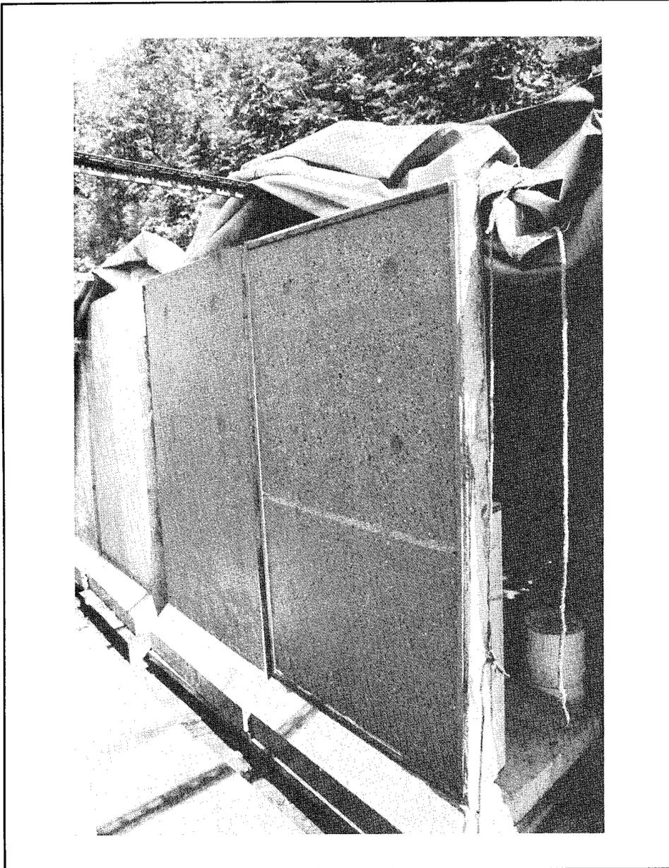
Figure 34. Panel application trial for repair material
