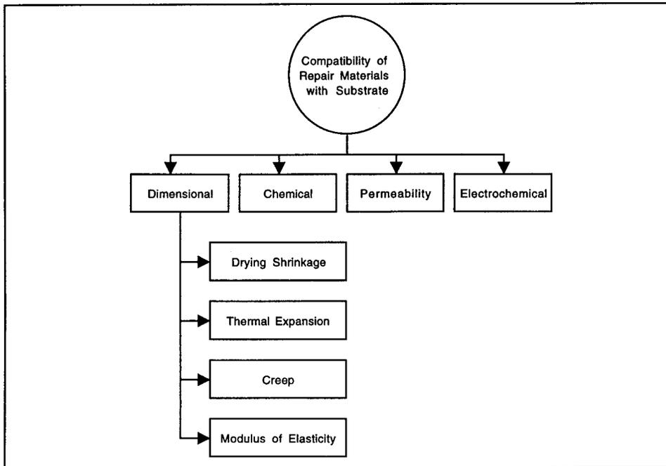
Figure 6. Factors affecting compatibility of repair materials
