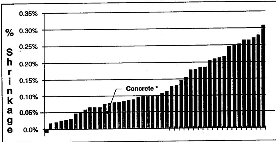
Figure 38. Alberta shrinkage test results
