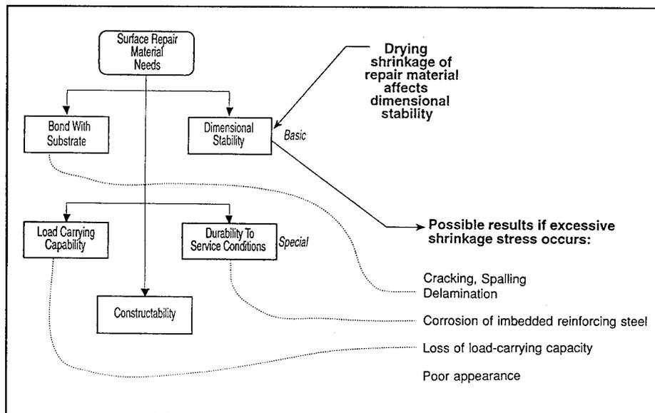
Figure 5. Surface repair material needs
