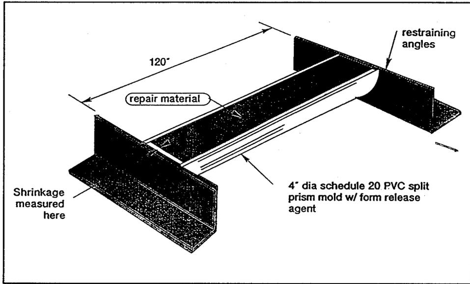
Figure 18. General view of the SPS test assembly
