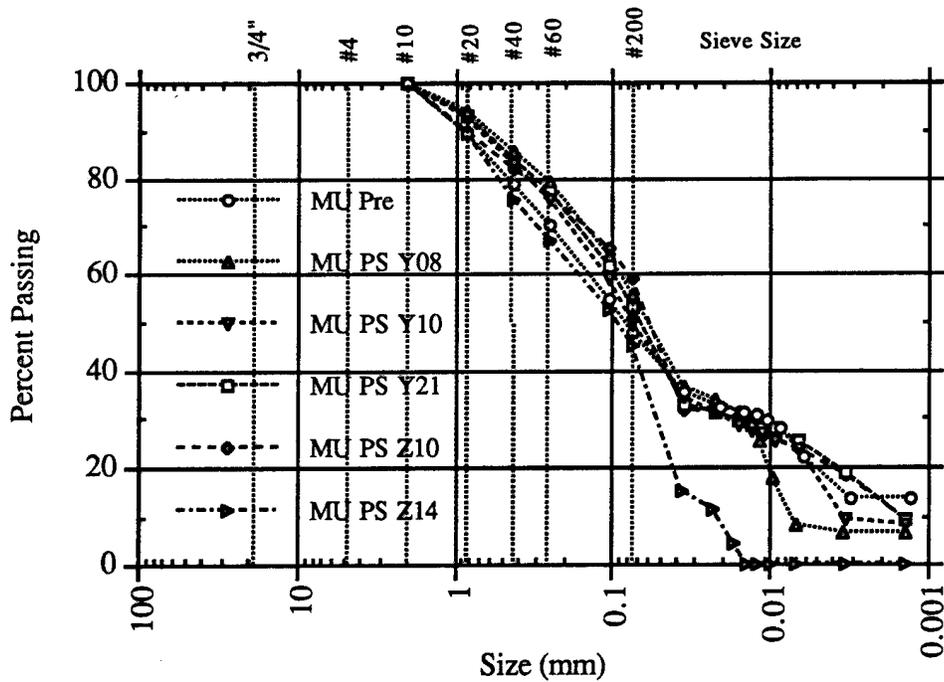
Figure A-16. MINOR UNCLE pre-test and all post-test ejecta gradations.
