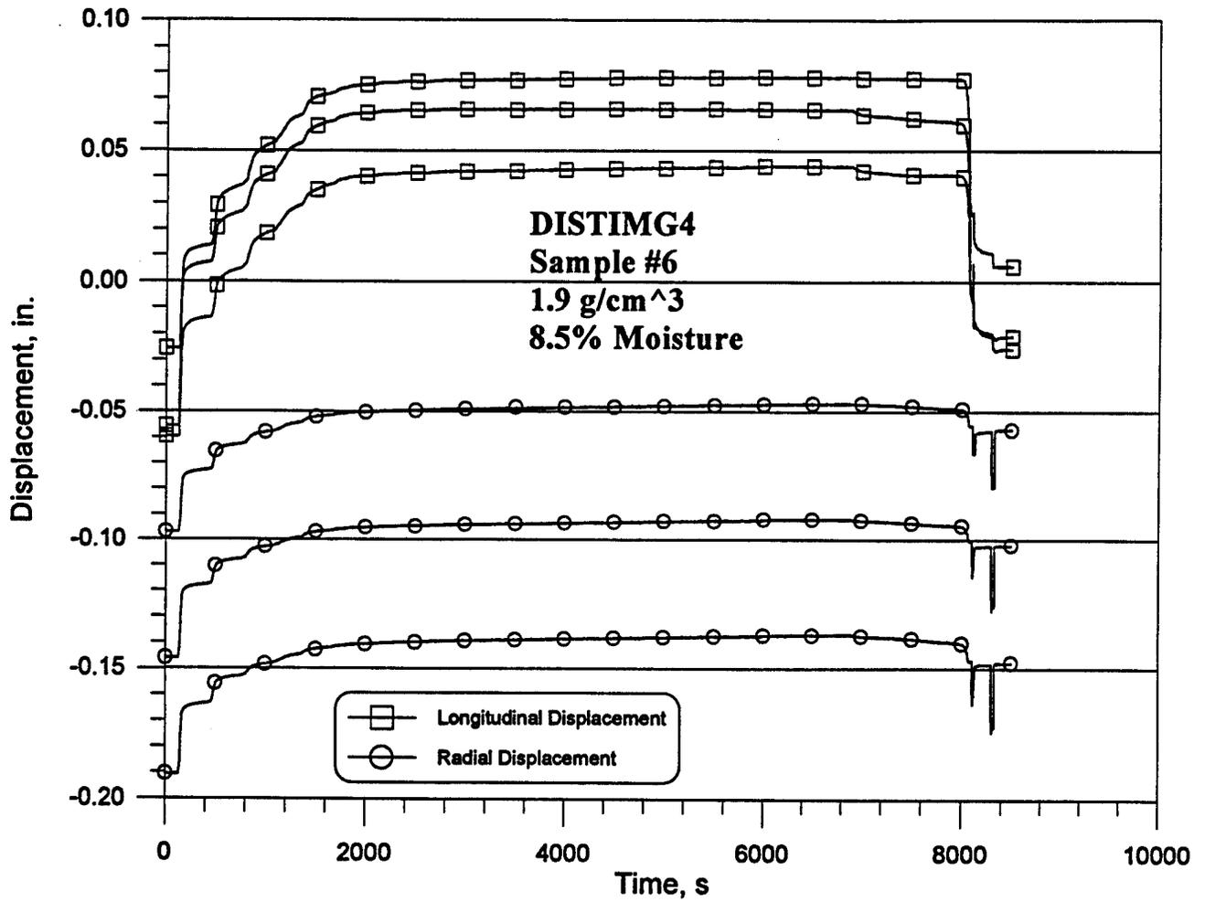
Figure B-20. Displacement time histories for test DISTIMG4.
