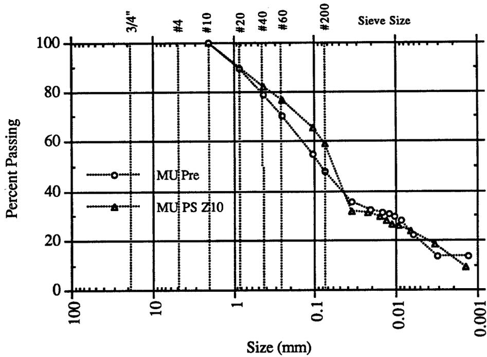
Figure A-14. MINOR UNCLE pre-test and post-test ejecta Z10 gradations.
