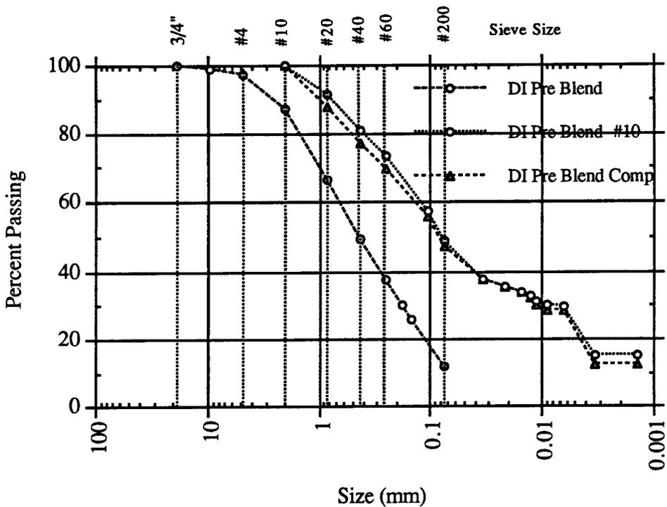
Figure A-2. DISTANT IMAGE pre-test and compacted sample gradations.
