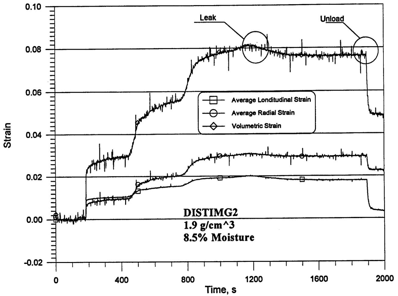
Figure B-9. Strain time histories for test DISTIMG2.
