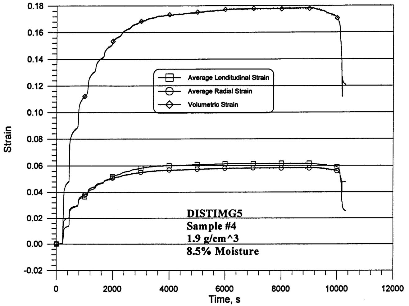
Figure B-29. Strain time histories for test DISTIMG5.
