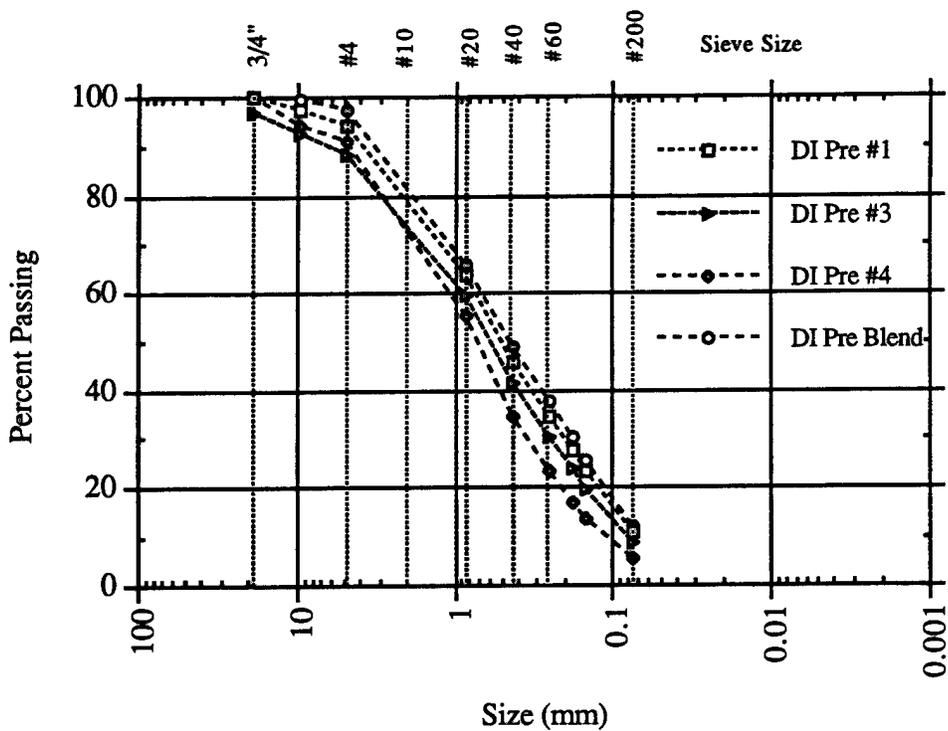
Figure A-1. DISTANT IMAGE pre-test and blend sample gradations.
