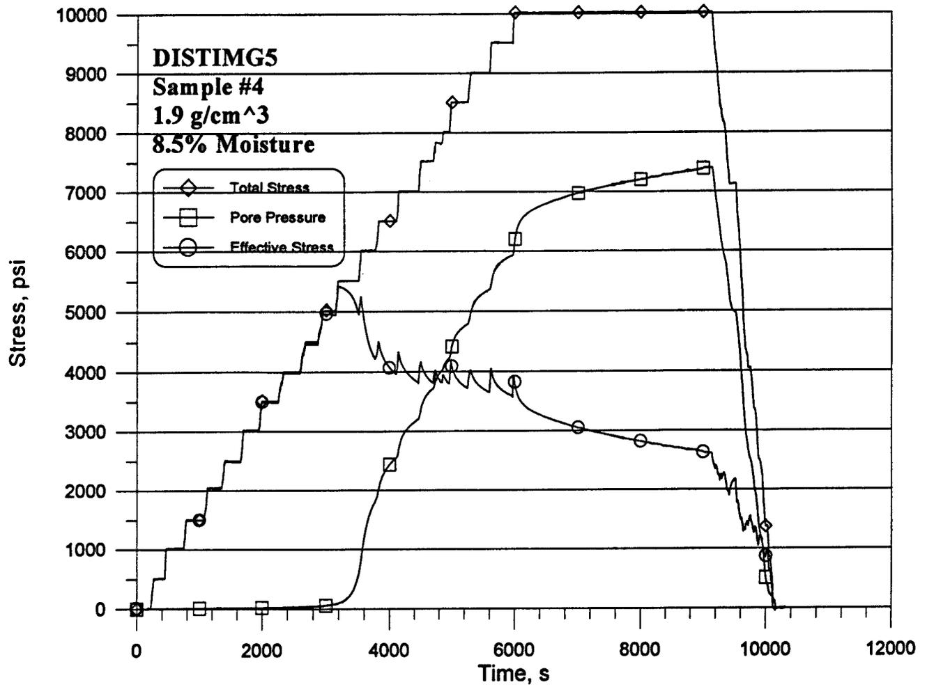
Figure B-27. Total stress, pore pressure, and effective stress time histories for test DISTING5.
