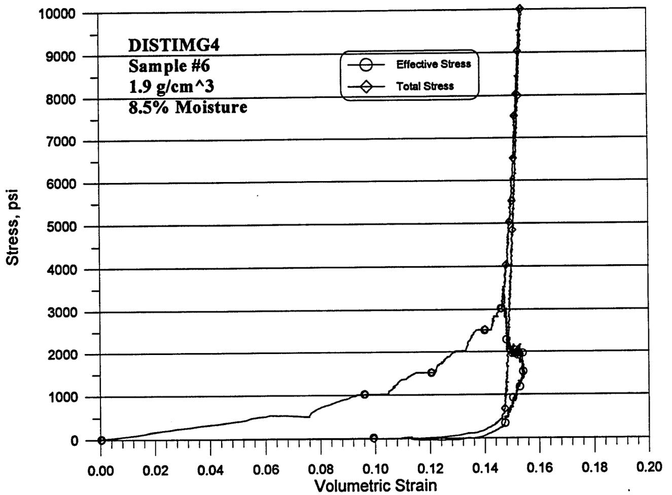
Figure B-22. Stress versus volumetric strain for test DISTIMG4.
