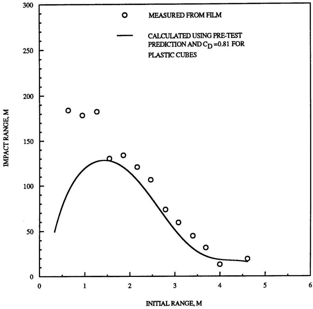
Figure 3-6. Comparison of calculated and measured impact ranges for plastic implants on HUSKY JAGUAR 2.
