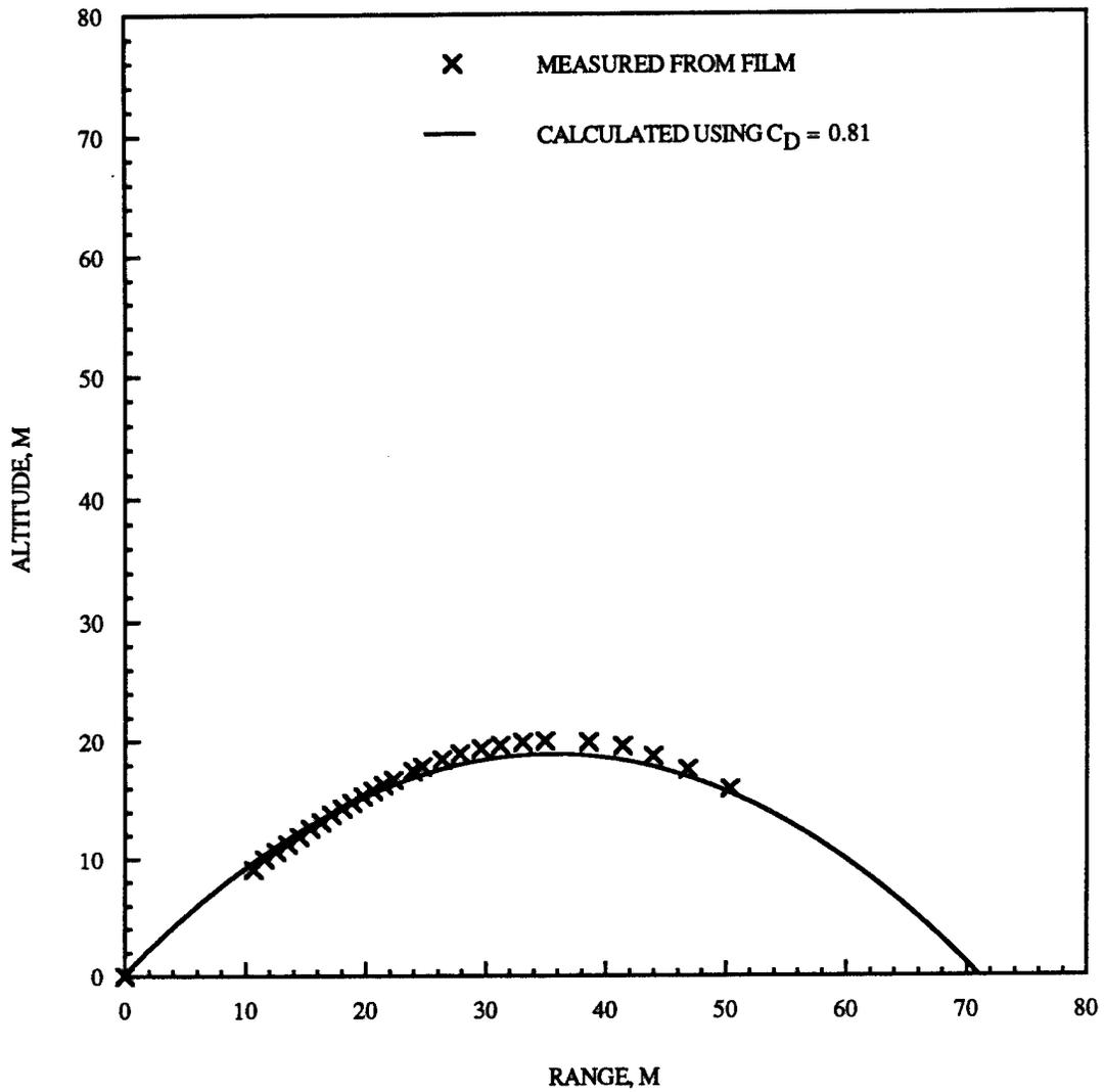
Figure 3-2. Comparison of calculated trajectory with trajectory 18 from film analysis for HUSKY JAGUAR 2.
