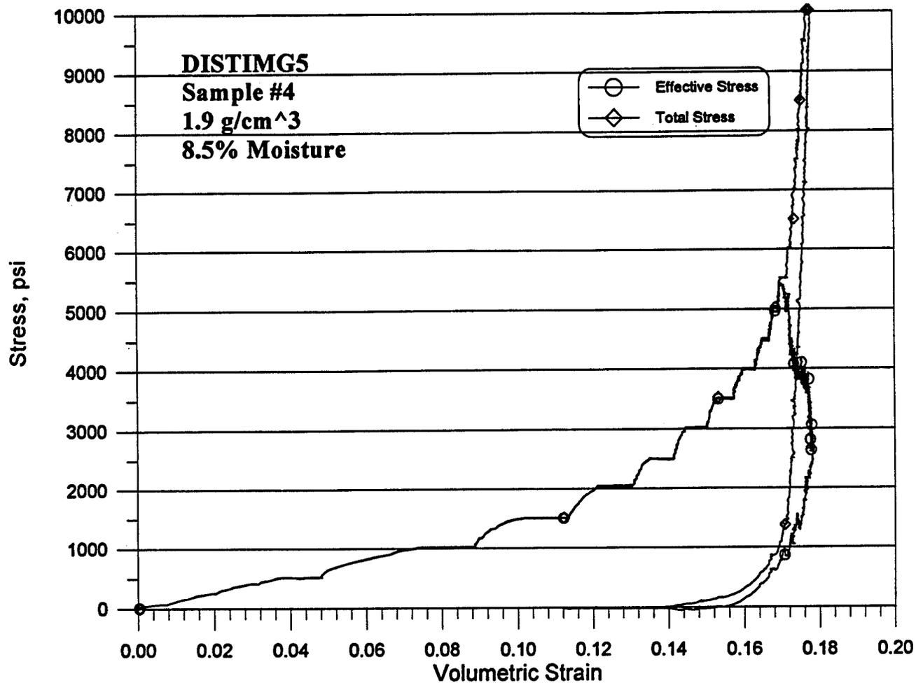
Figure B-30. Stress versus volumetric strain for test DISTIMG5.
