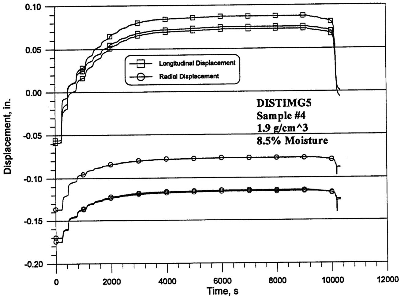
Figure B-28. Displacement time histories for test DISTIMG5.
