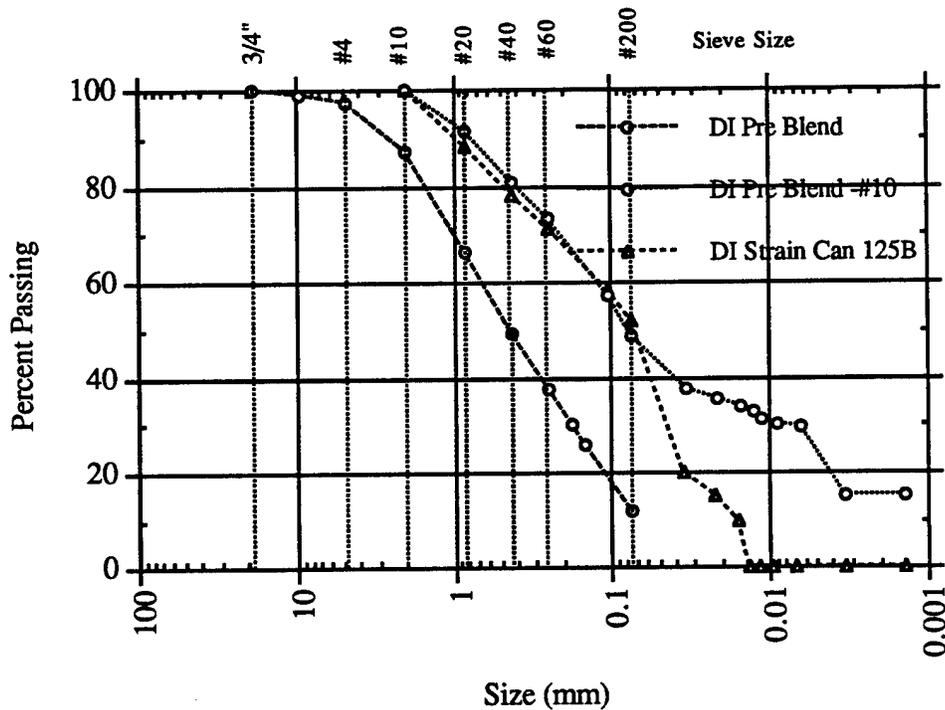
Figure A-8. DISTANT IMAGE pre blend and Strain Can 125B gradations.
