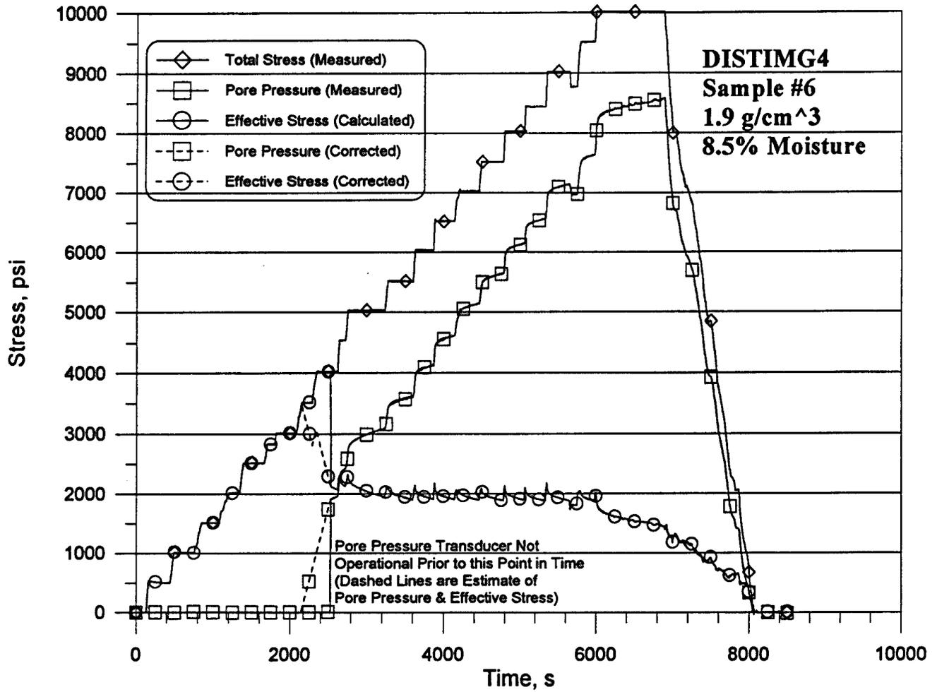
Figure B-19. Total stress, pore pressure, and effective stress time histories for test DISTIMG4.
