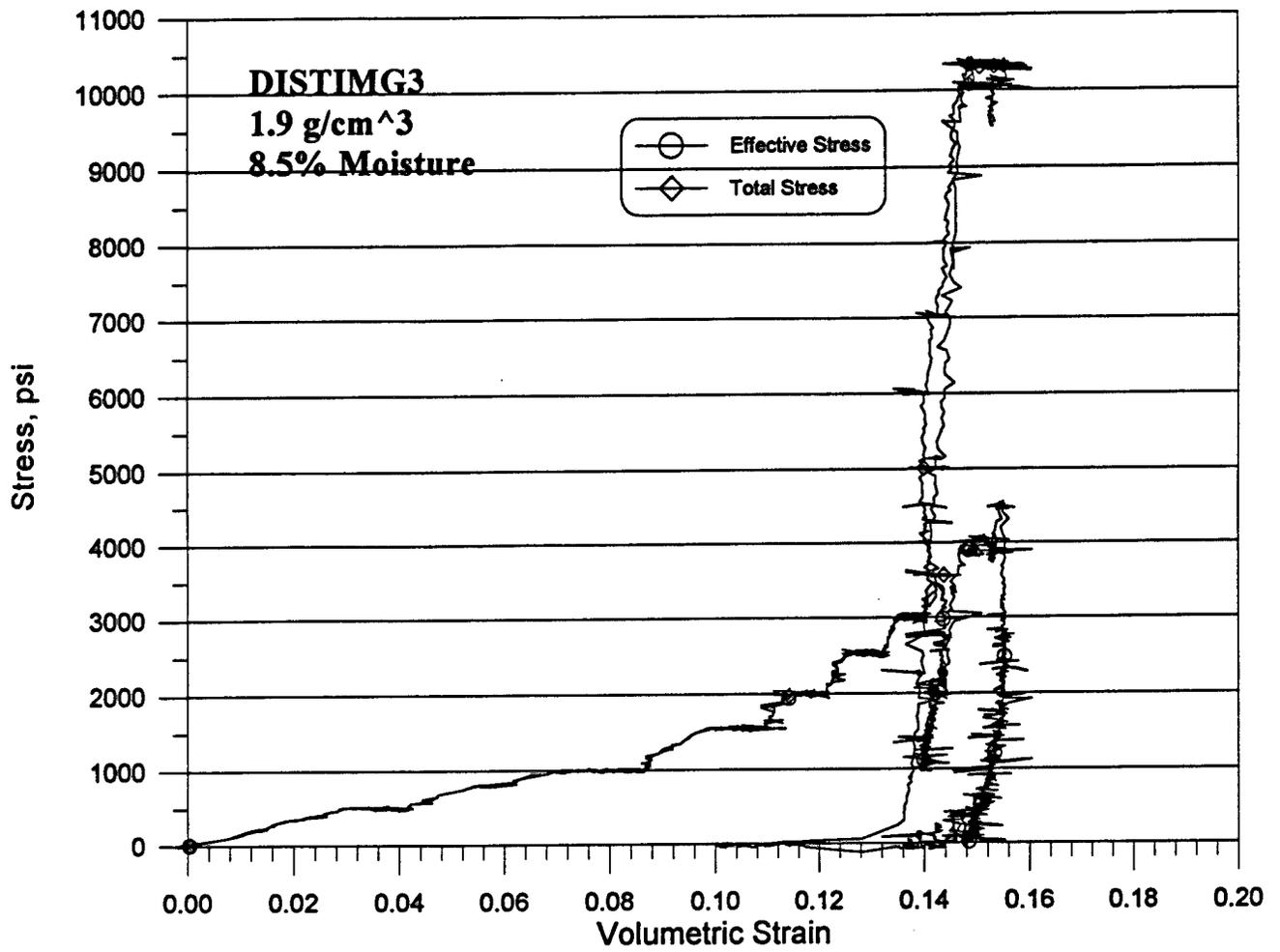
Figure B-16. Stress versus volumetric strain for test DISTIMG3.
