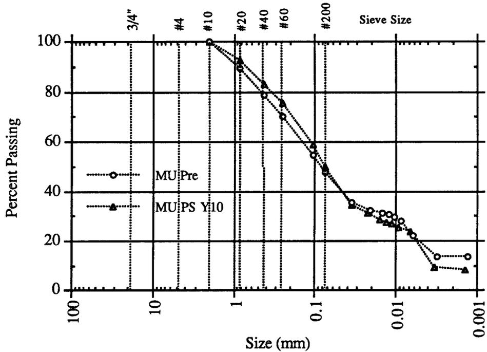
Figure A-12. MINOR UNCLE pre-test and post-test ejecta Y10 gradations.
