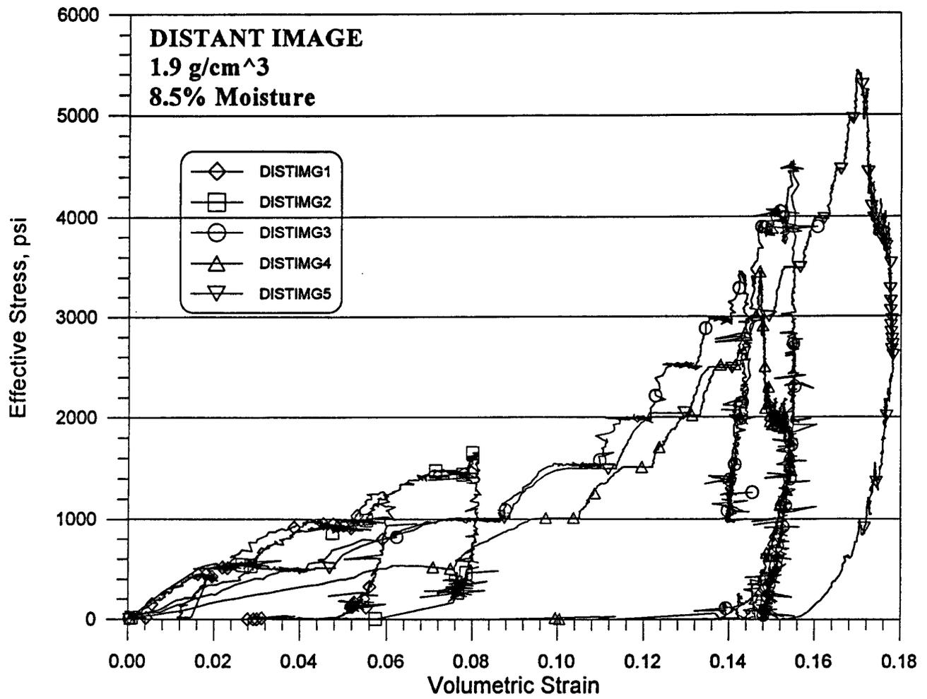
Figure B-35. Summary of effective stress versus volumetric strain for five tests.
