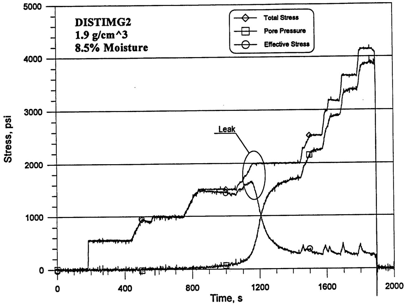
Figure B-7. Total stress, pore pressure, and effective stress time histories for test DISTIMG2.
