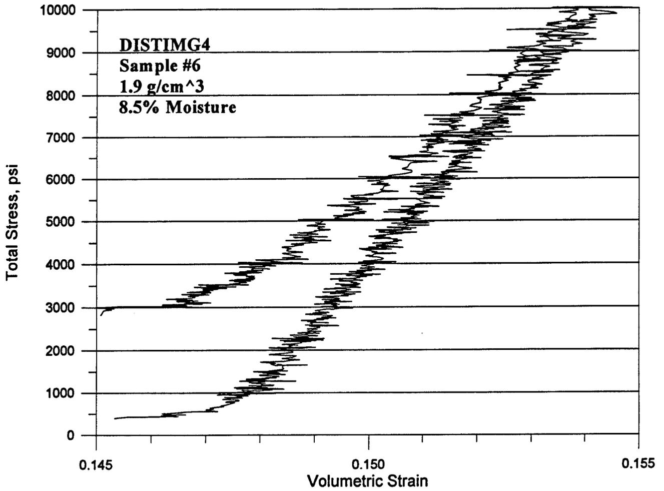
Figure B-25. Total stress versus volumetric strain for test DISTIMG4 (detail).
