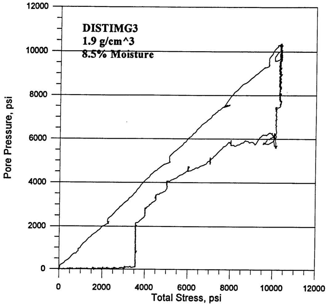
Figure B-18. Pore pressure versus total stress for test DISTIMG3.
