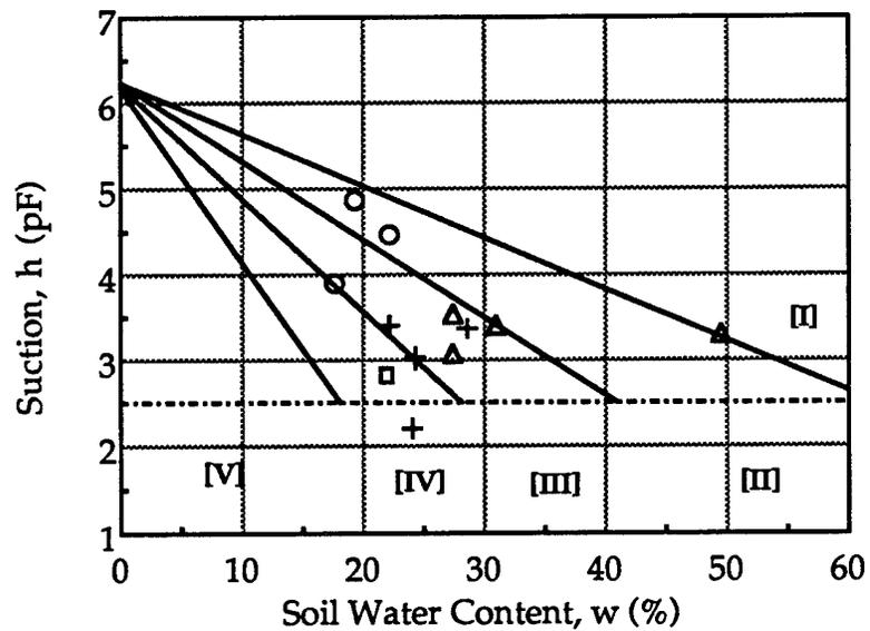
Figure A-20. Expansive soil classification system (McKeen 1992).
