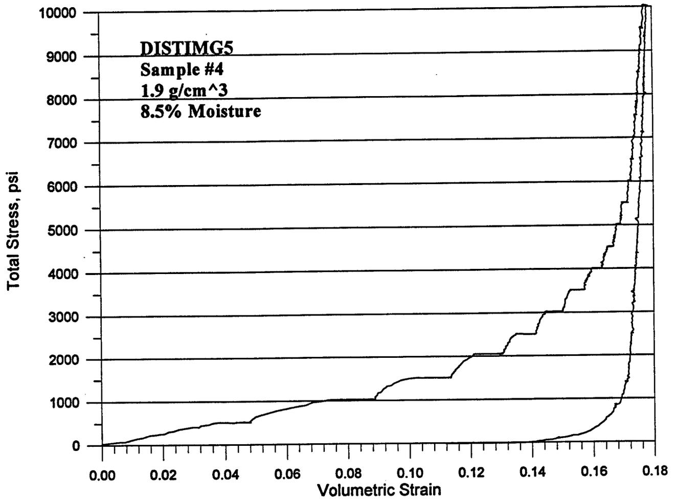
Figure B-32. Total stress versus volumetric strain for test DISTIMG5.
