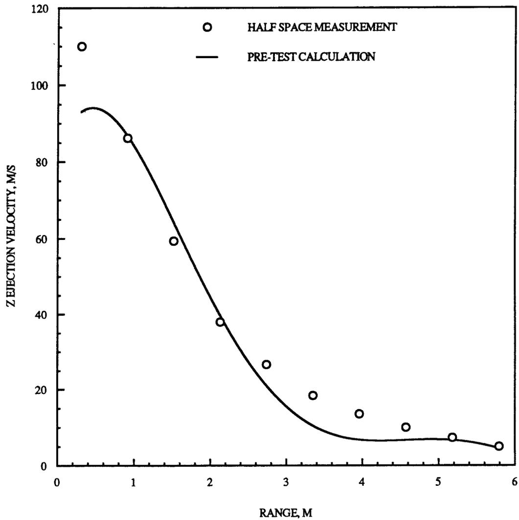
Figure 5-4. Comparison of vertical velocity component from pre-test calculation to measurements from halfspace test for HUSKY JAGUAR 2.
