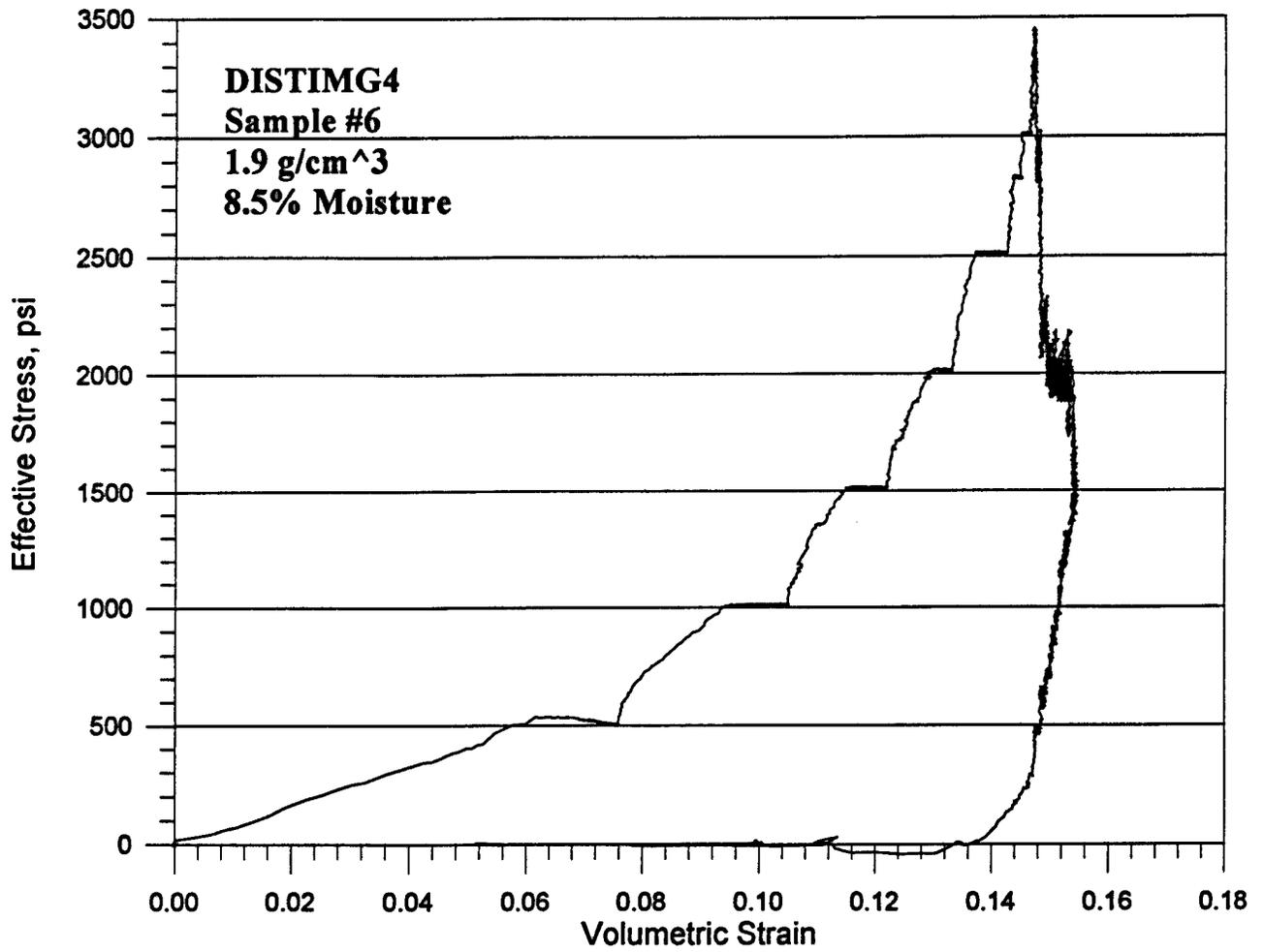
Figure B-23. Effective stress versus volumetric strain for test DISTIMG4.
