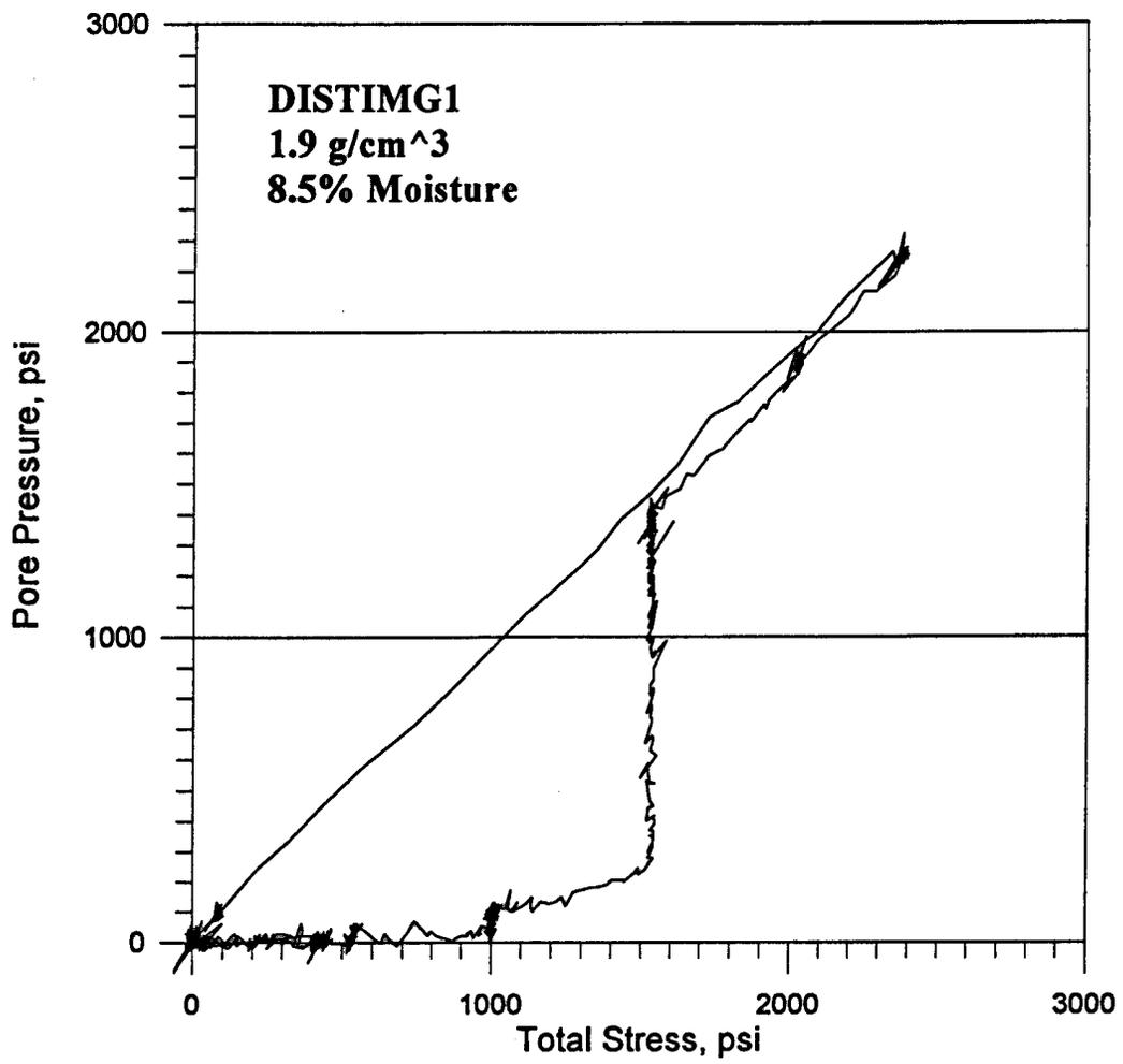
Figure B-6. Pore pressure versus total stress for test DISTIMG1.
