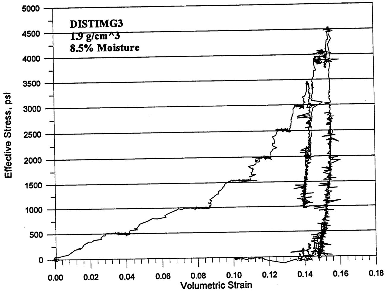
Figure B-17. Effective stress versus volumetric strain for test DISTIMG3.
