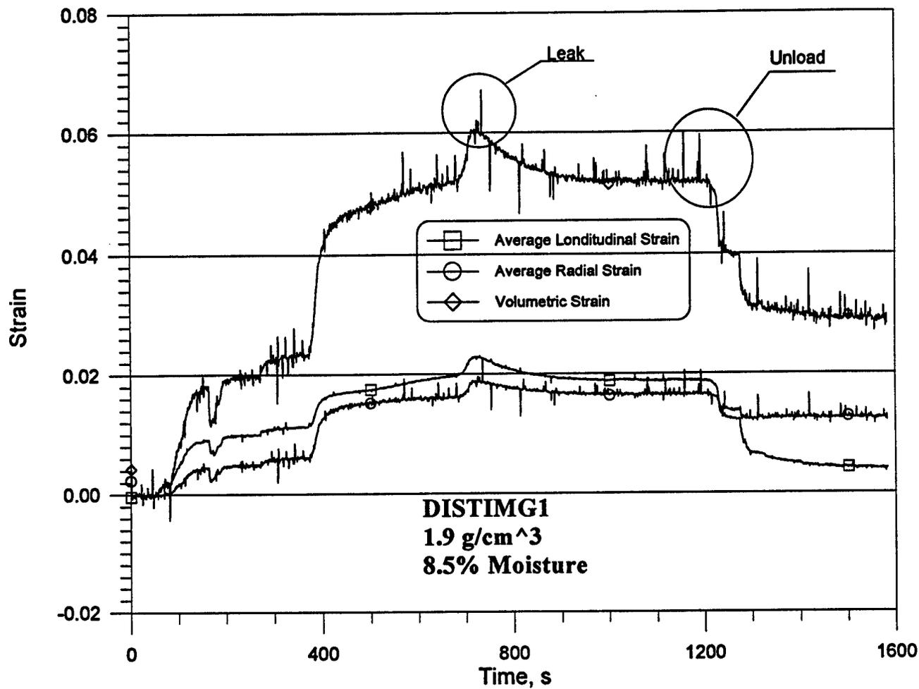
Figure B-3. Strain time histories for test DISTING1.
