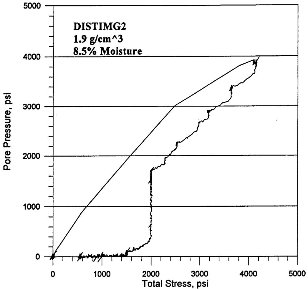
Figure B-12. Pore pressure versus total stress for test DISTIMG2.
