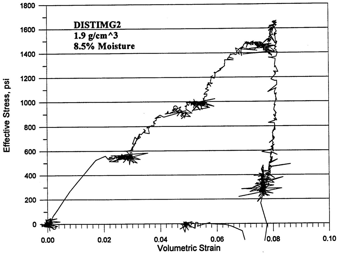
Figure B-11. Effective stress versus volumetric strain for test DISTIMG2.
