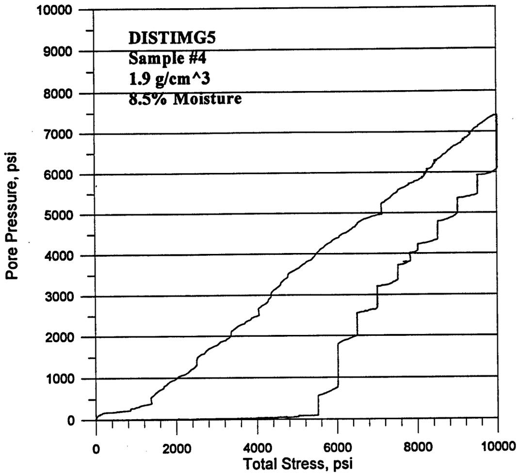
Figure B-34. Pore pressure versus total stress for test DISTIMG5.
