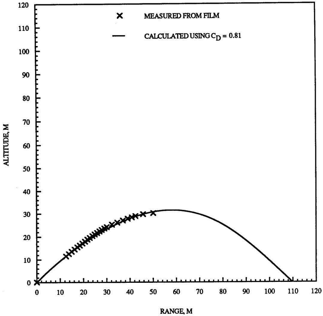
Figure 3-3. Comparison of calculated trajectory with trajectory 20 from film analysis for HUSKY JAGUAR 2.
