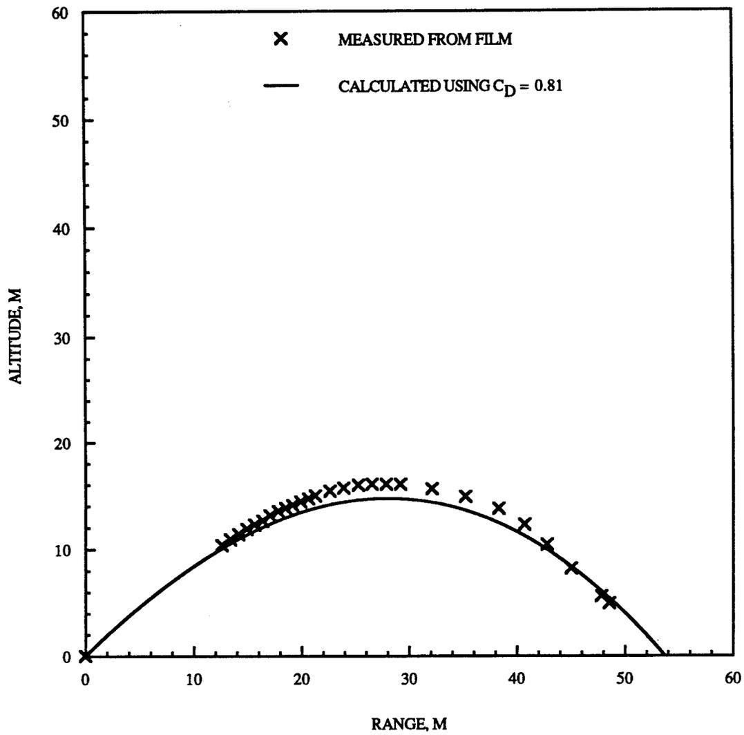
Figure 3-1. Comparison of calculated trajectory with trajectory 25 from film analysis for HUSKY JAGUAR 2.
