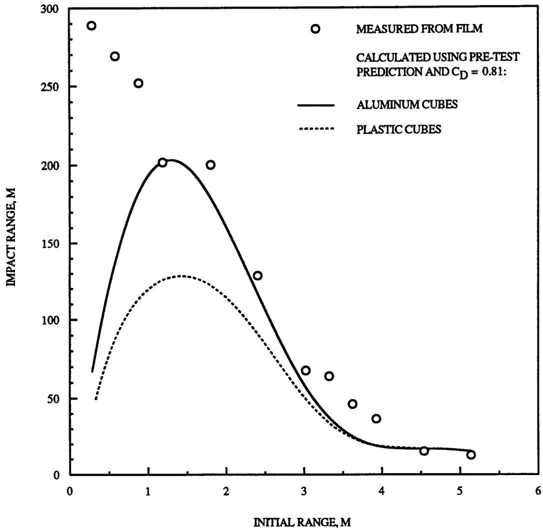
Figure 3-5. Comparison of calculated and measured impact ranges for aluminum implants on HUSKY JAGUAR 2.
