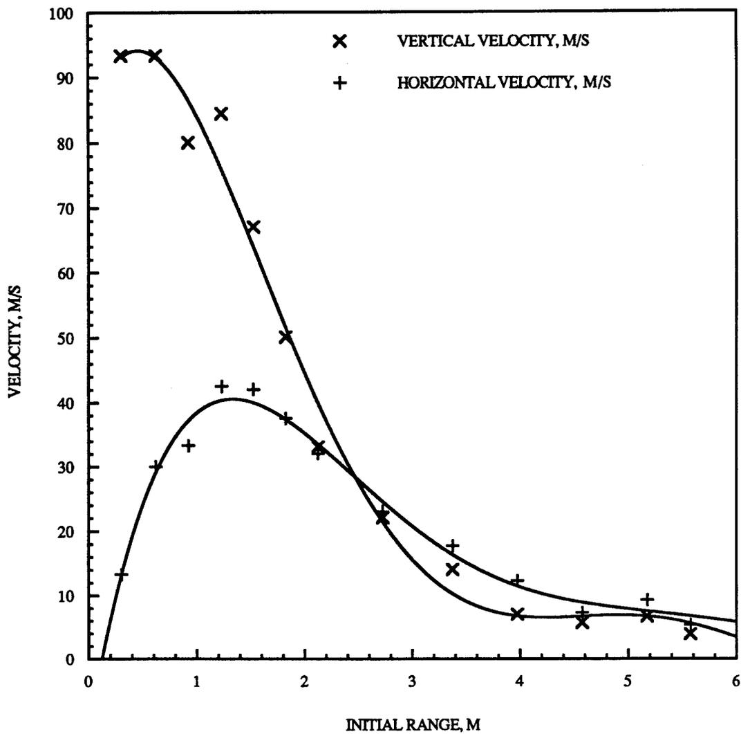
Figure 3-4. Ejection velocity components from pre-test prediction for surface soil layer for HUSKY JAGUAR 2.
