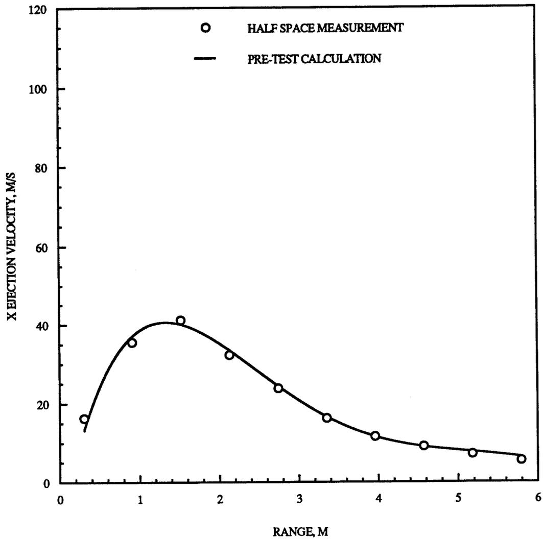
Figure 5-3. Comparison of horizontal velocity component from pre-test calculation to measurements from halfspace test for HUSKY JAGUAR 2.
