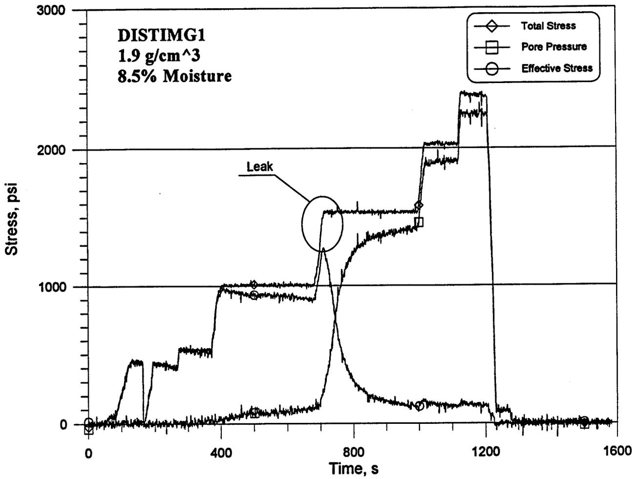
Figure B-1. Total stress, pore pressure, and effective stress time histories for test DISTING1.
