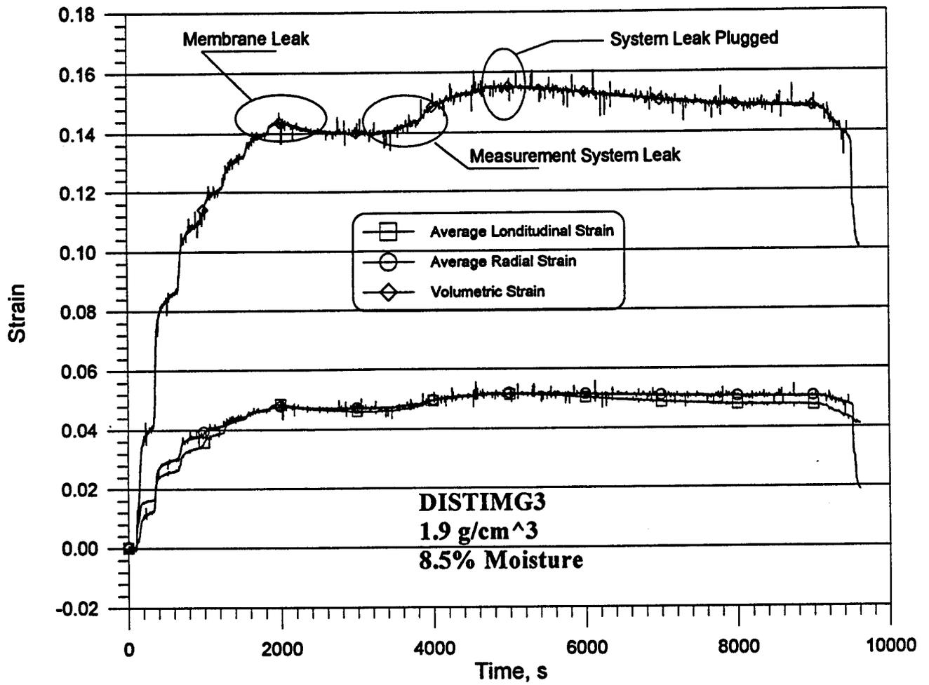
Figure B-15. Strain time histories for test DISTIMG3.
