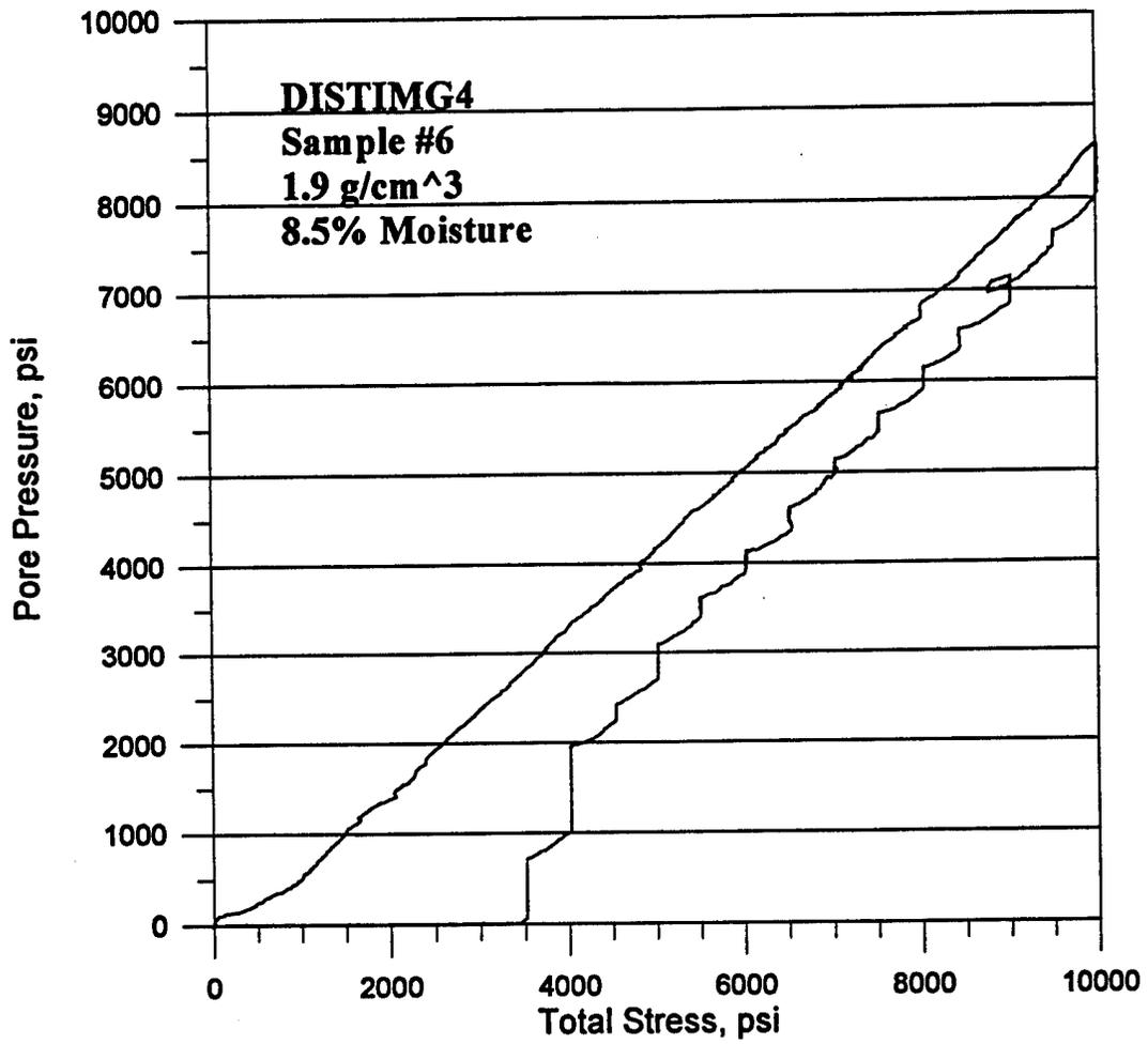
Figure B-26. Pore pressure versus total stress for test DISTIMG4.
