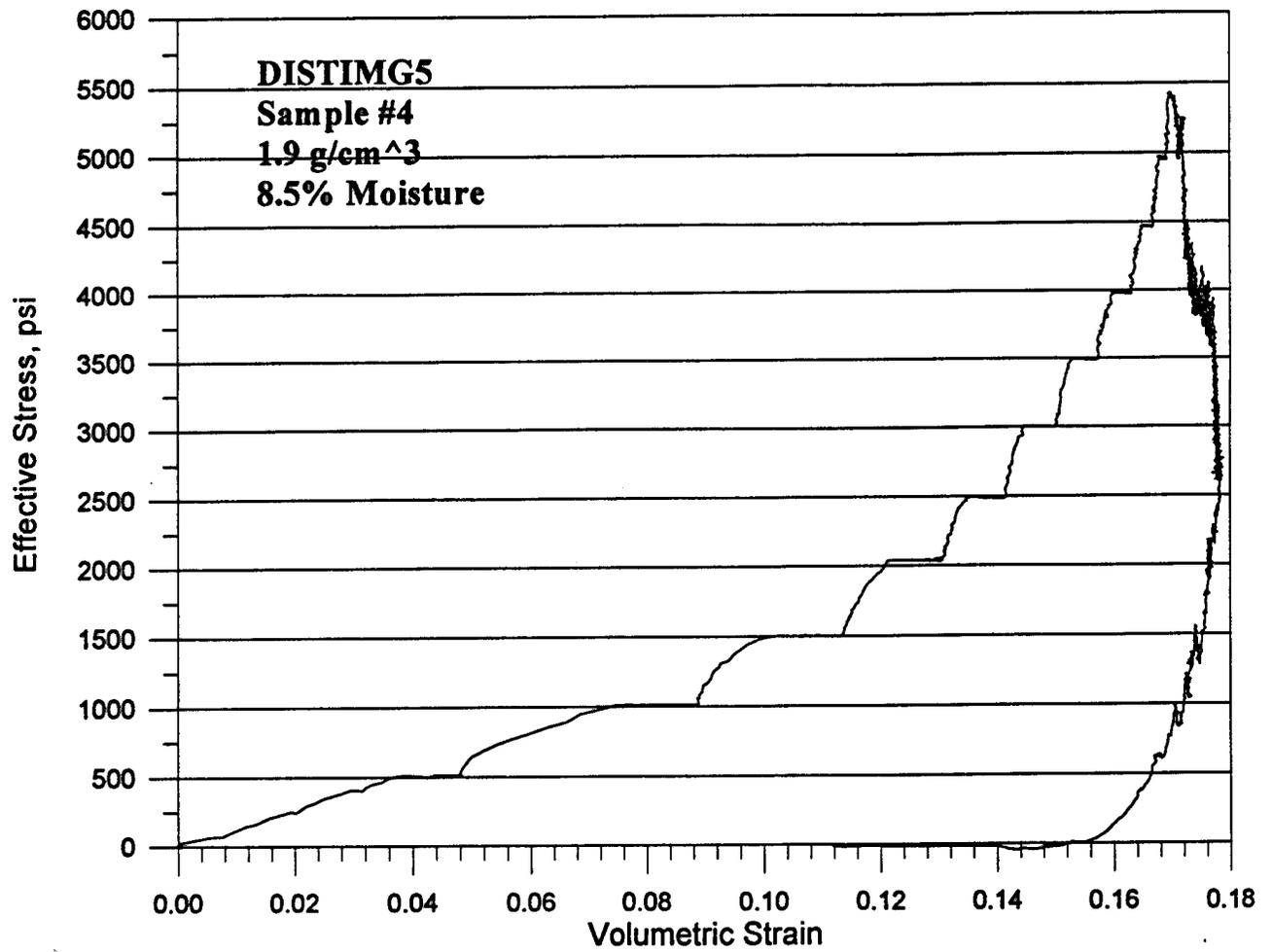
Figure B-31. Effective stress versus volumetric strain for test DISTIMG5.
