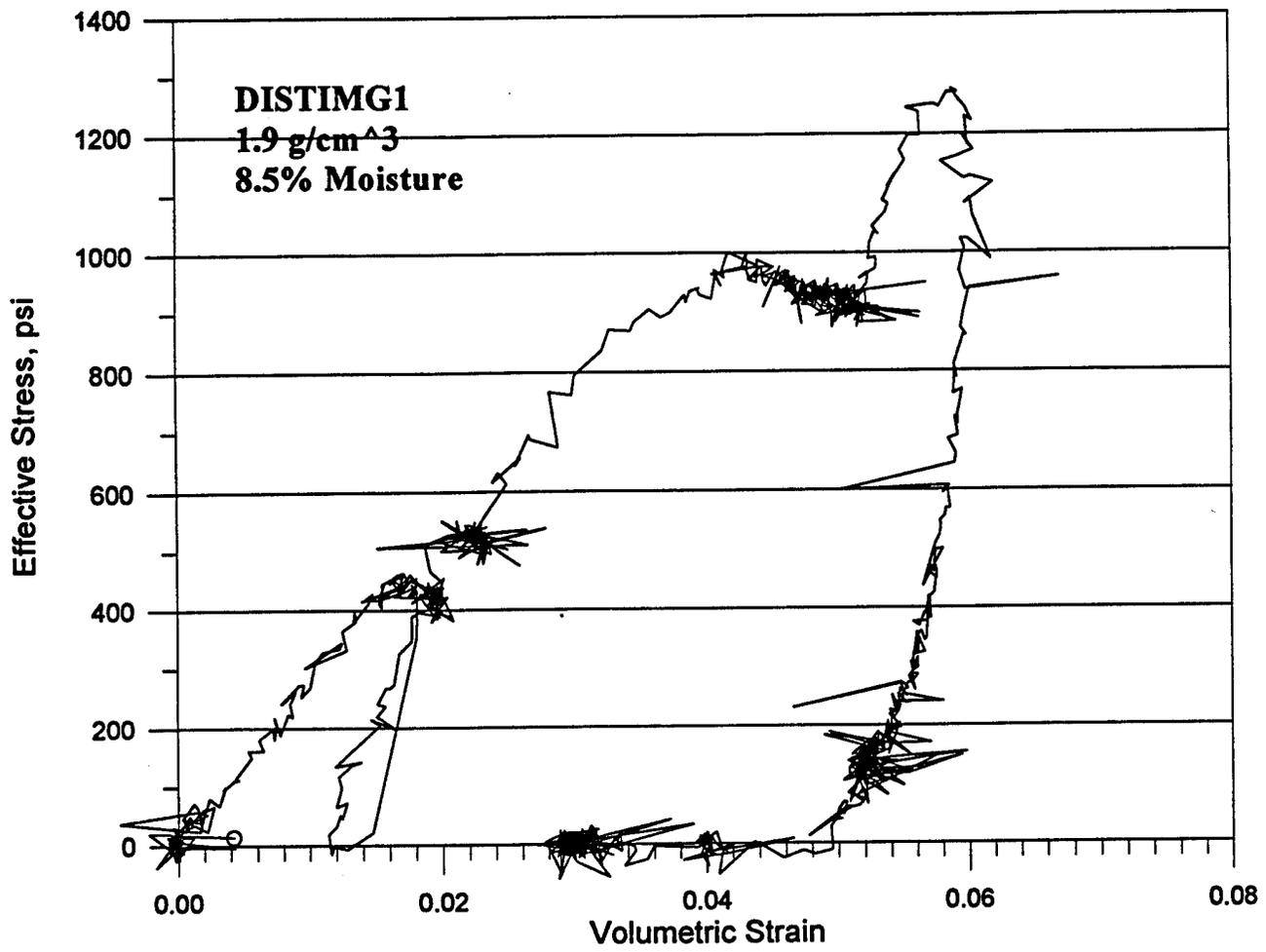
Figure B-5. Effective stress versus volumetric strain for test DISTIMG1.
