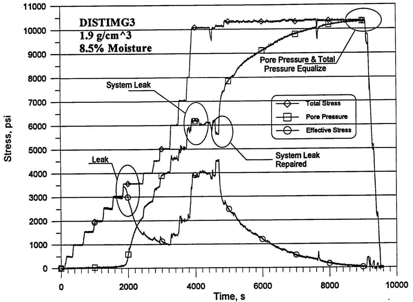
Figure B-13. Total stress, pore pressure, and effective stress time histories for test DISTIMG3.
