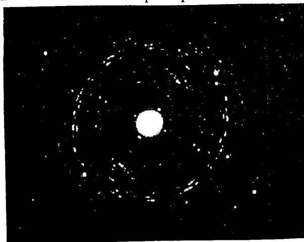
Figure 9. TED from an \text{Ir}_3\text{Si}_4 film deposited at ambient and reacted at 450 °C to form a silicide.
