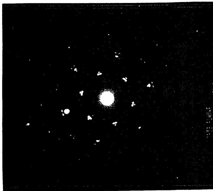
Figure 13 . TED pattern displaying the highly oriented \text{Ir}_3\text{Si}_4 crystallite growth formed by depositing Ir on Si(111) at 500 °C.
