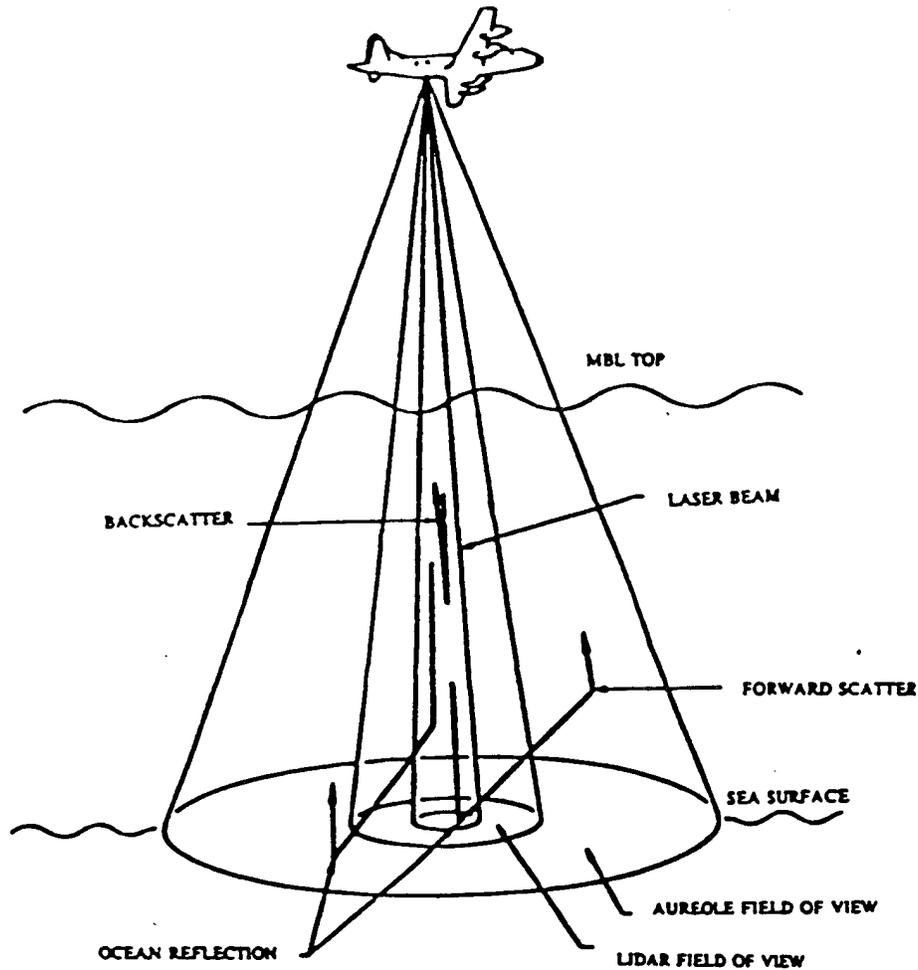
**Figure 21.** Signal paths of the lidar and aureole signal.
