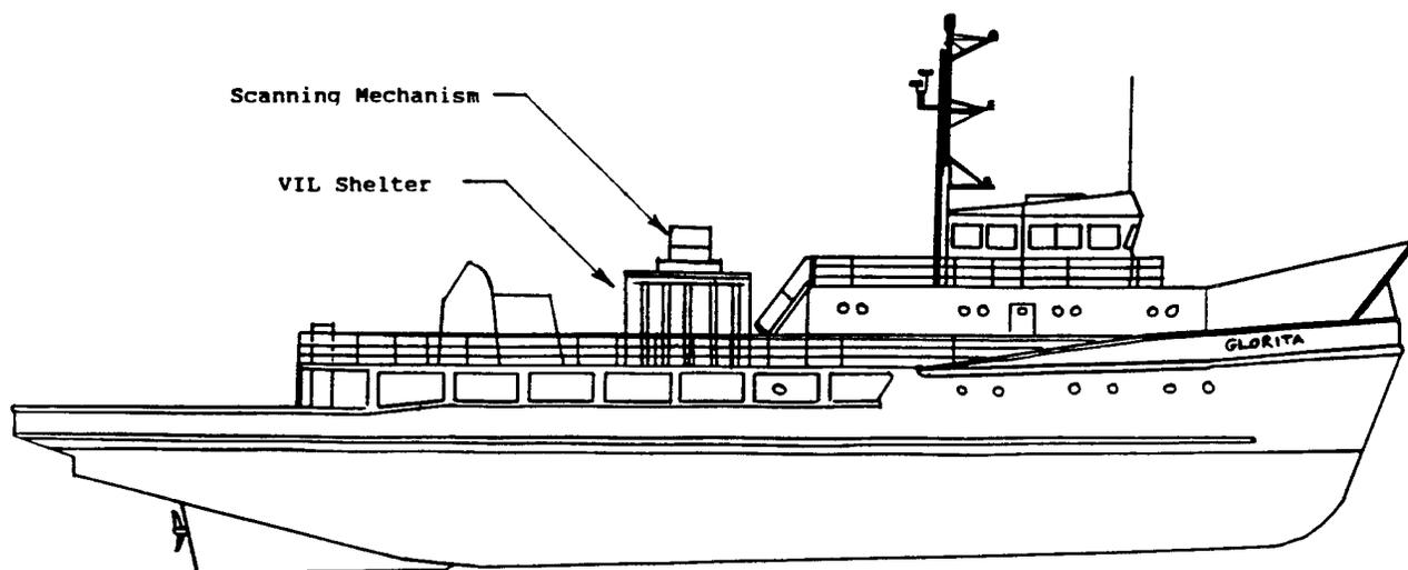
**Figure 15.** Shipboard configuration of the VIL.
