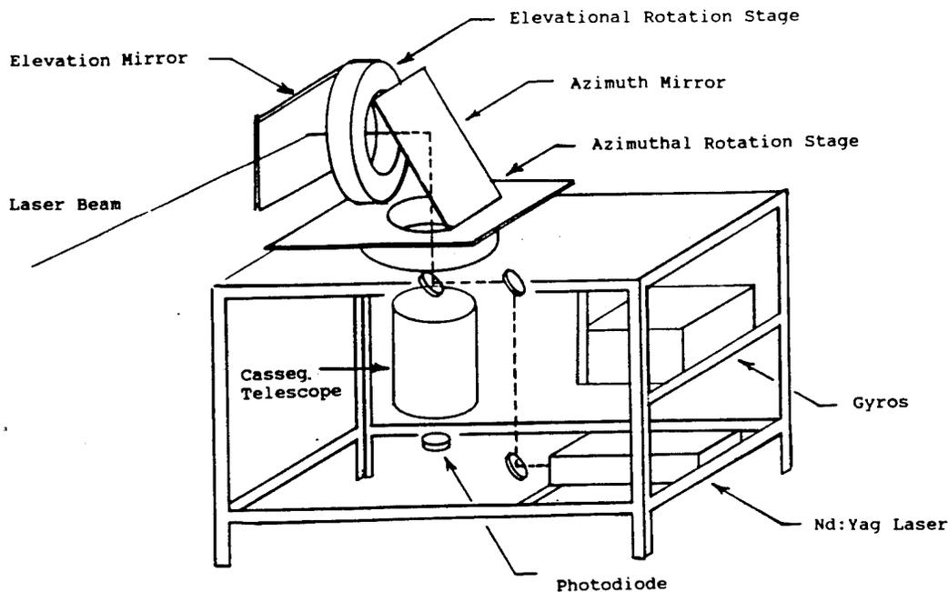
**Figure 8.** Scanning system layout.
