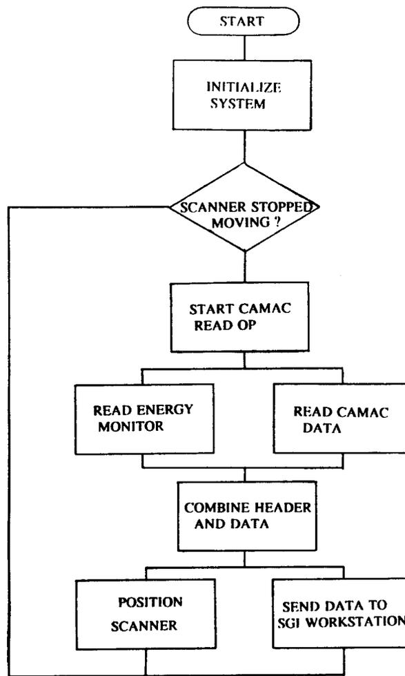
**Figure 13.** Order of events during the data acquisition cycle.
