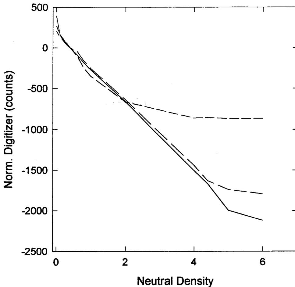
**Figure 26.** The relationship between digitizer counts and neutral density filter is shown. Curves for three topographic targets are plotted. The strength of the topographic targets are from strongest to weakest, using line types of solid, long dash, and short dash, respectively. The curves are normalized by a neutral density filter of 0.2 and the counts are therefore negative.
