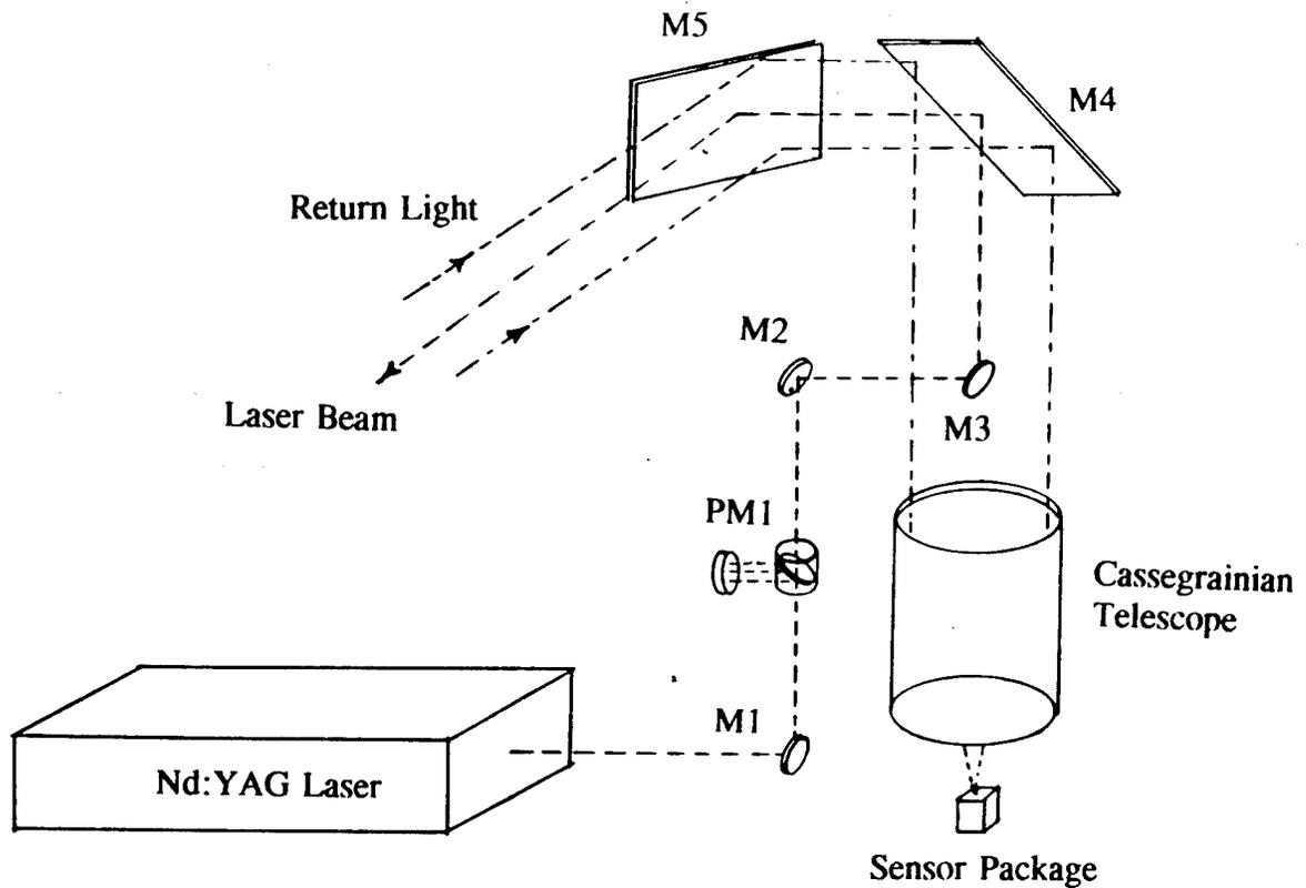
Figure 9. Laser beam transmission path.
