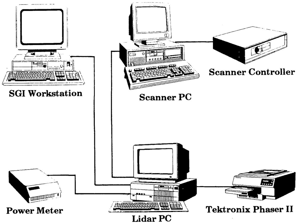
**Figure 19.** VIL computer interconnections during shipboard use.
