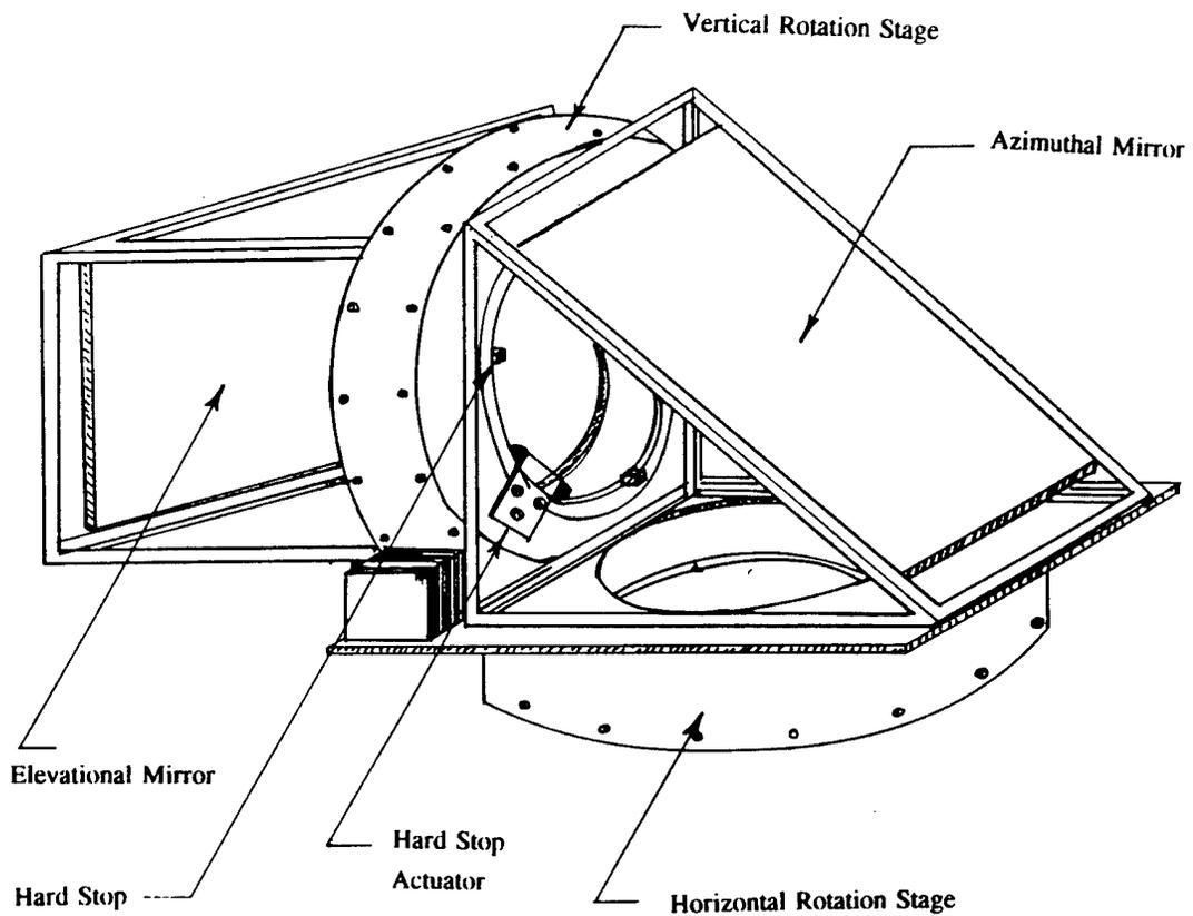
**Figure 6.** Description of the VIL scanning mechanism.
