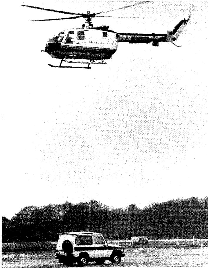
Figure 16 : Position Hold Flight Test Arrangement
