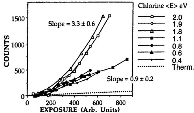
Fig. 12 Total etch product ( $\text{SiCl}_3^+$ ) as a function of exposure and energy.
