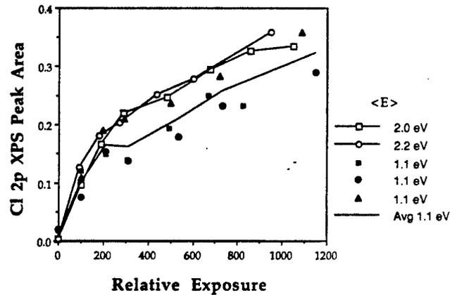
Fig. 11 XPS signal from Cl 2p following exposure at different energies.
