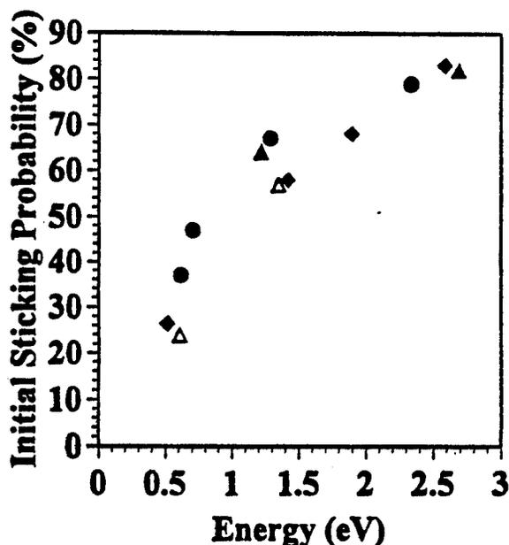
Fig. 14 Upper limit of  $\text{Cl}_2$  and Cl sticking probabilities ( $S_0$ ) vs. kinetic energy. (●) and (◆) Two different runs using velocity-selected kinetic energies of  $\text{Cl}_2$ . (▲) Two different average energies using the full kinetic energy distribution of  $\text{Cl}_2$  (not velocity selected). (△) Two different average energies of Cl atom using the full kinetic energy distribution (not velocity selected).
