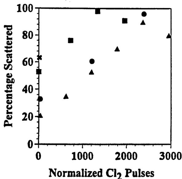
**Fig. 13** Percentage of scattered  $\text{Cl}_2$  as a function of incident beam energy. (✖)  $\langle E \rangle = 0.6$  eV. (■)  $\langle E \rangle = 0.71$  eV. (●)  $\langle E \rangle = 1.3$  eV. (▲)  $\langle E \rangle = 2.59$  eV. Increased exposure with number of pulses of the unchopped beam indicate that the percent scattered increases with coverage.
