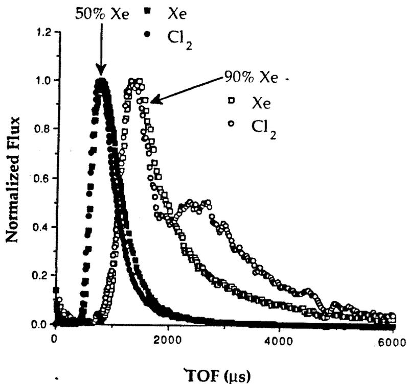
Fig. 7 time-of-flight traces for Xe and Cl<sub>2</sub> from laser-vaporized mixtures.
