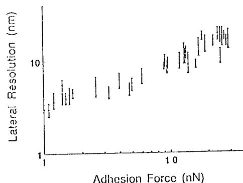
Fig. 14 Adhesion force vs lateral resolution.
