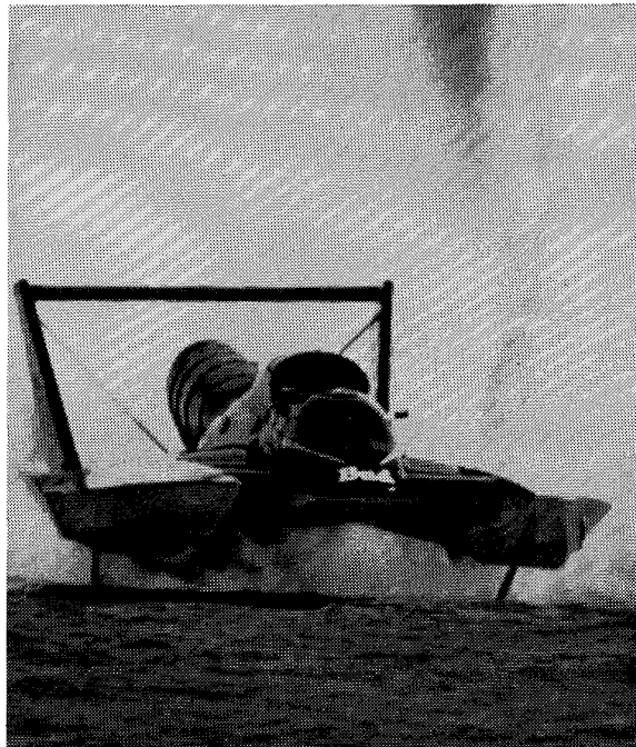
Figure 3 - Current Unlimited-Class Racing Hydroplane Operating at Speed in Ground Effect (Ref. 4)
