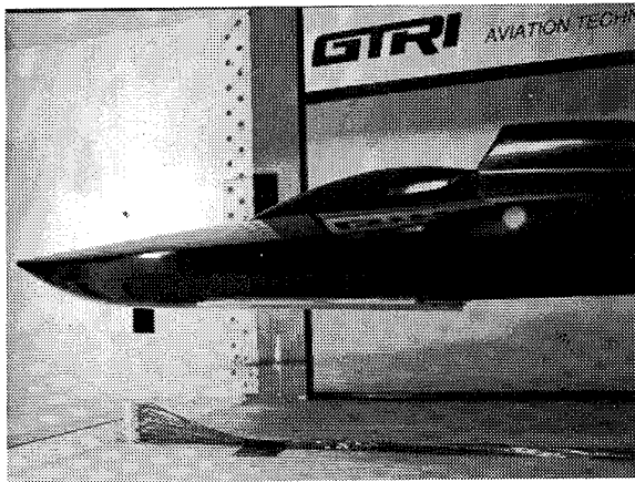
Figure 7 - Hydroplane Installation, Showing Boundary-Layer Probe and Tangential Floor-Blowing Slot at Test Section Entrance (x=0.0")
