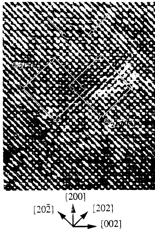
Fig. 7. Experimental HREM image of a [001](100) edge dislocation in Fe-50Al. Note how the \{220\} extra half planes terminate approximately 10-12 atom positions apart on the slip plane possibly indicating a glide dissociation.
