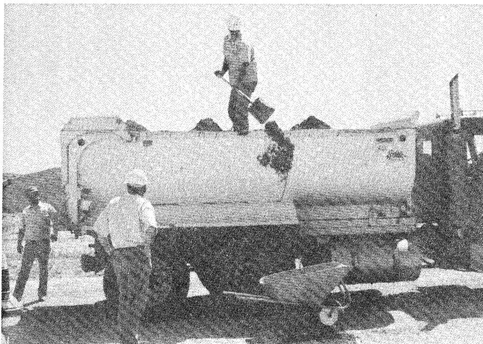
Photo E3. Concrete being removed from the dump truck for specimen making
