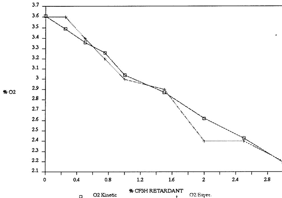
**Figure 13:** %O<sub>2</sub> as CF<sub>3</sub>H concentration increases.
