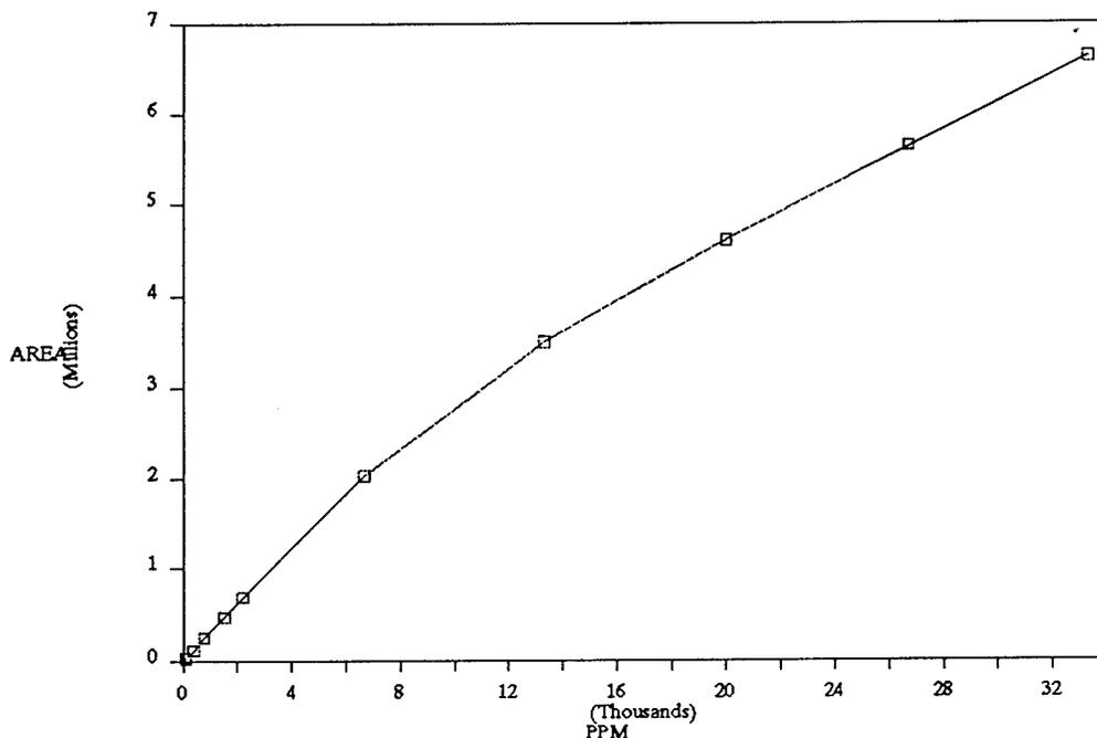
Figure 18: CF<sub>3</sub>Br GC-FID Calibration Graph
