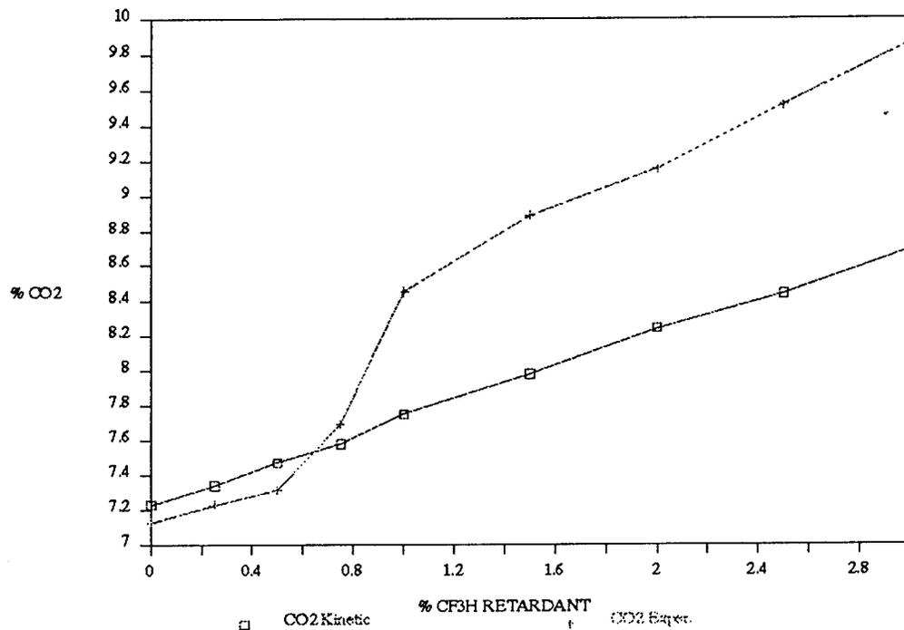
Figure 14: %CO<sub>2</sub> as CF<sub>3</sub>H concentration increases.
