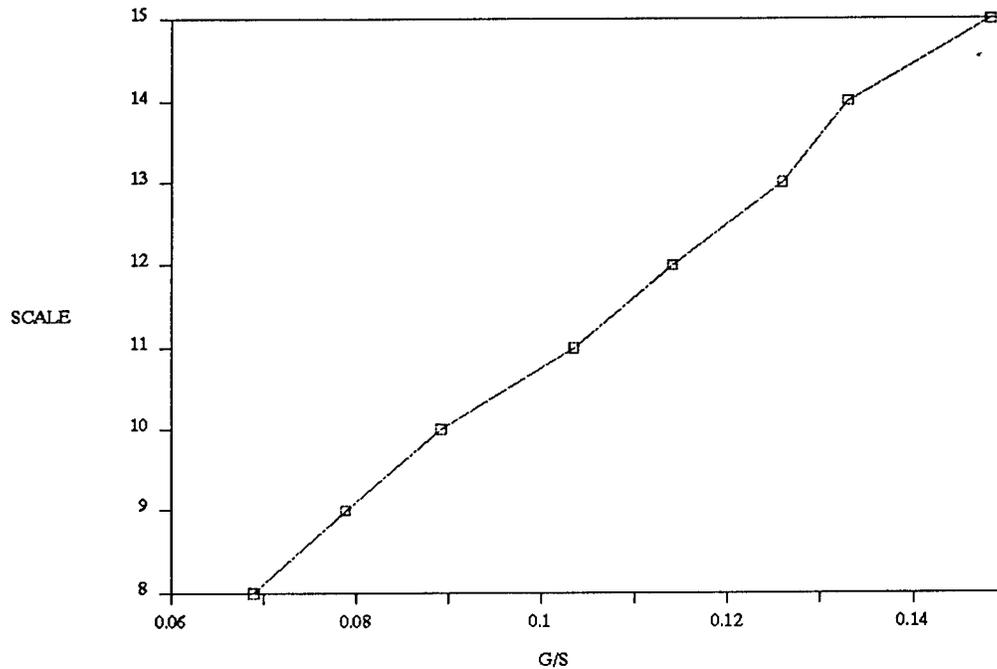
Figure 15: CF<sub>3</sub>Br Calibration Graph
