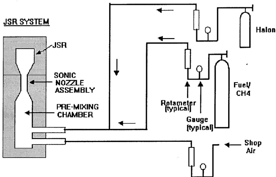
Figure 3: Fuel/Air/Halon Delivery System
