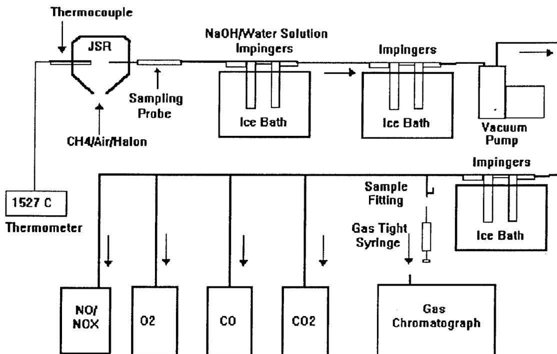
Figure 5: Modified Experimental System
