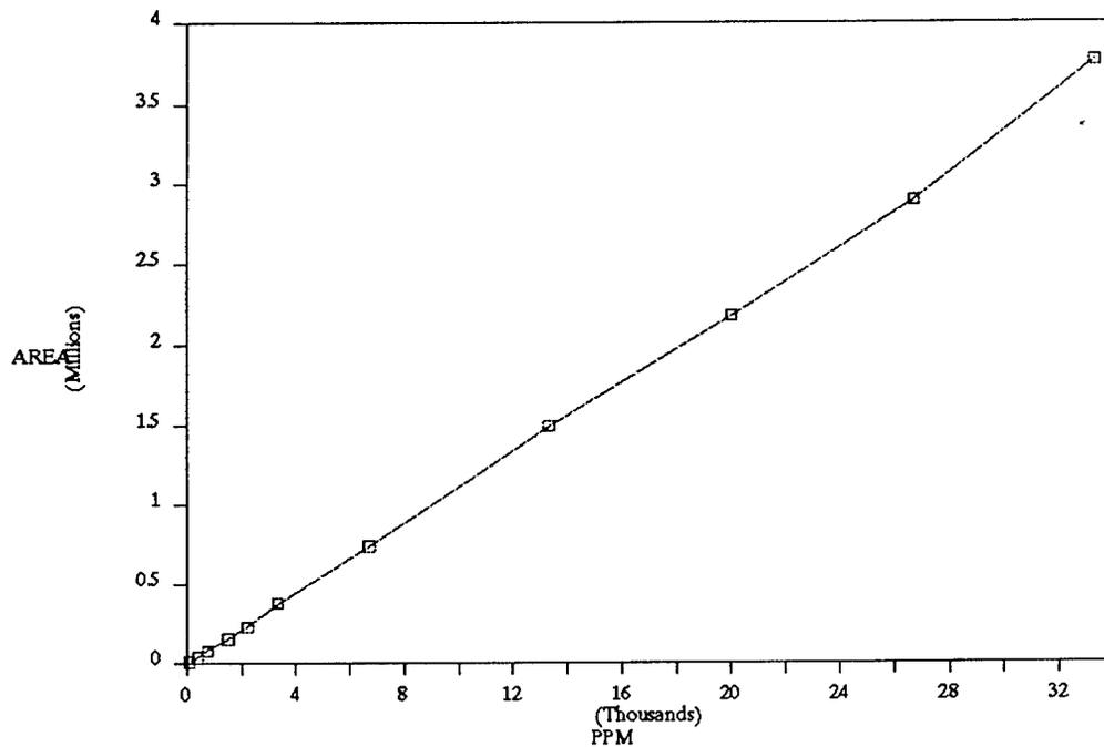
**Figure 19:** CF<sub>3</sub>H GC-FID Calibration Graph
