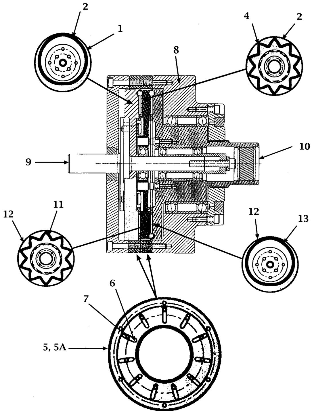
Figure 1.2.2-2: The basic multi-stage SYNKdrive.
