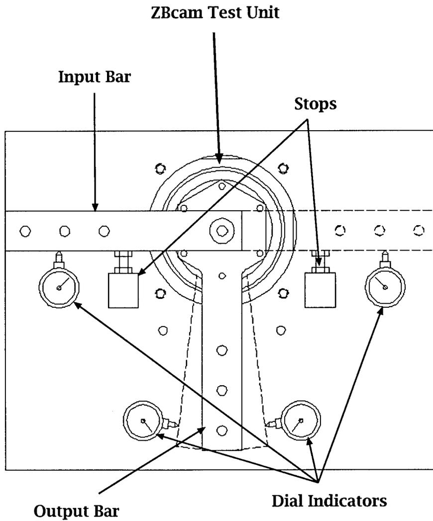
Figure 2.4.1.1-1: Prototype test assembly.
