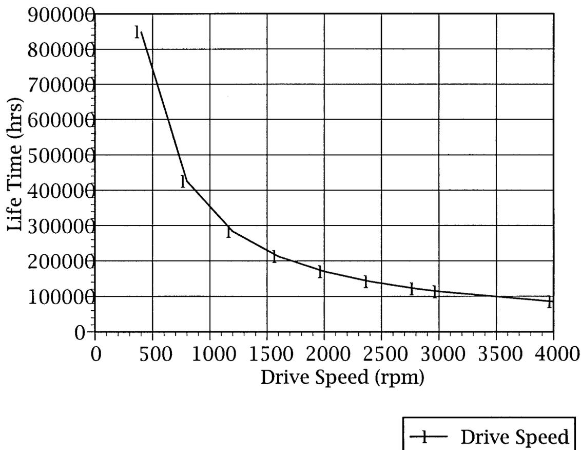
Figure 2.2.8-9: Load-life calculation for 52% conformity and 40% flank angle.
