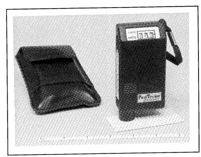
made of a durable, hardened plastic, the positector works when held normal (perpendicular) to any positioned surface. It is adjustable to unusual substrates, and the reading is unaffected by aging or reasonable shock, temperature, and vibration environments. Accessories—(0-60 mils) with tungsten carbide probe tip, 9-volt battery, set of sample thickness standards, and leather case.
