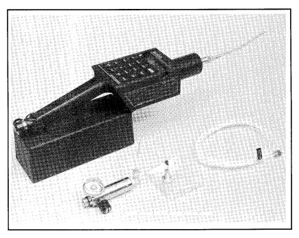
ple instructions and reading are visible on an LCD panel. Accessories—carrying case, calibration kit, analog cable, printer cable, three-meter sample line, and rechargeable snap-on battery pack.
