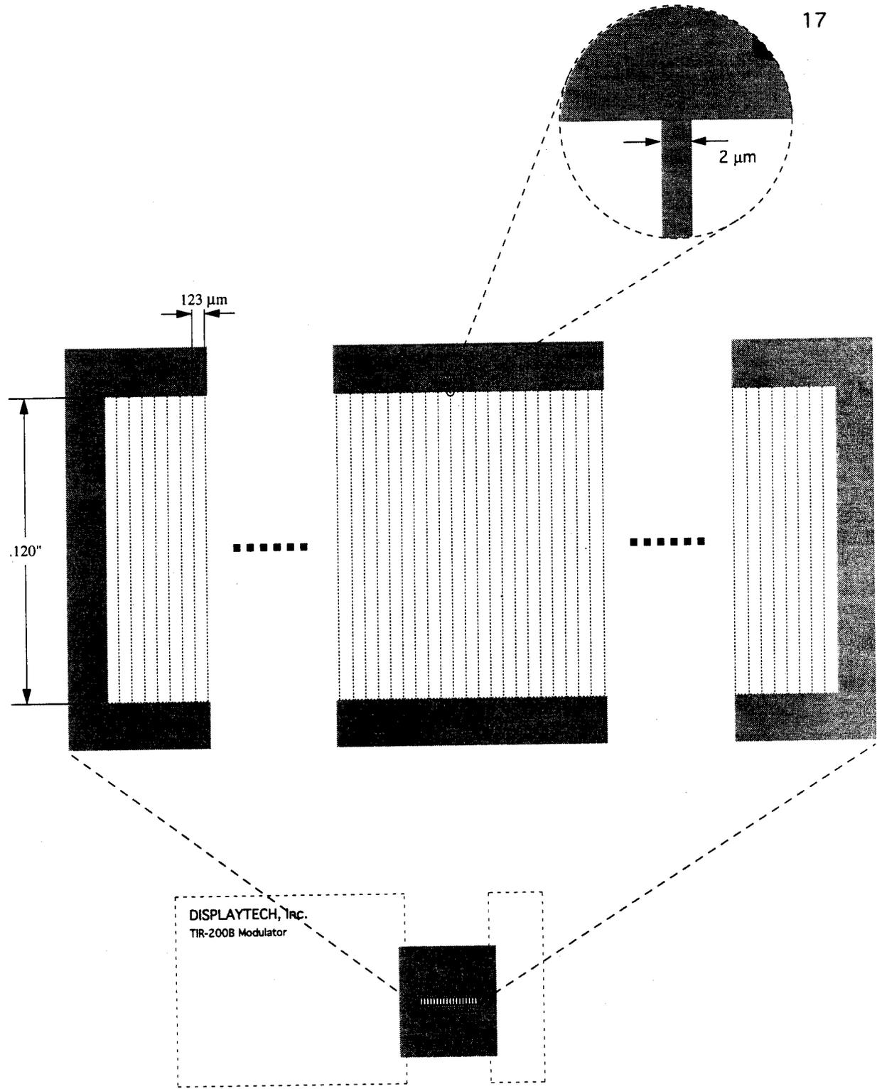
Figure 2.5.2: Pixel arrangement of the TIR SLM
