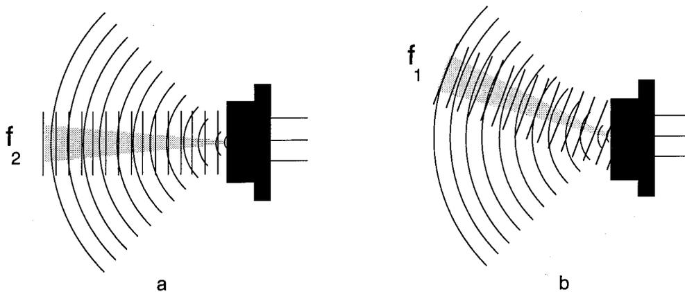
Figure 2.4.2: Sampling of acoustooptic aperture by heterodyne detection.
