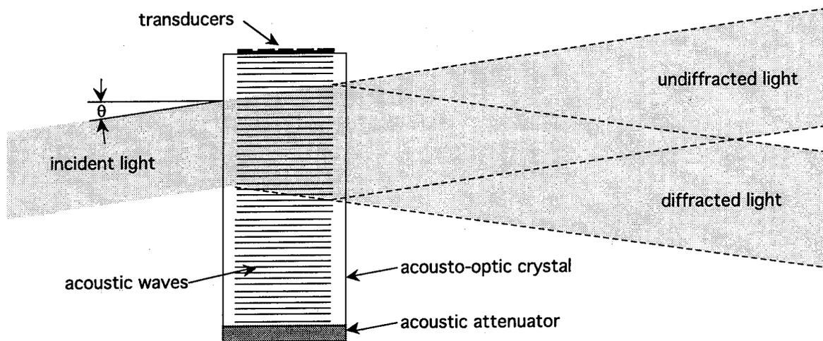
Figure 2.2.1: Acousto-optic Cell
