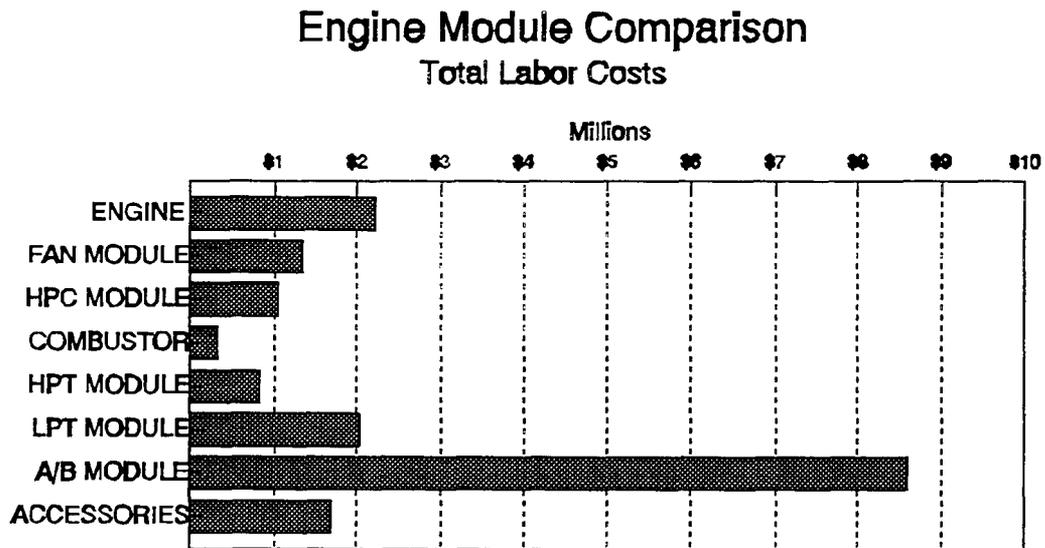
Figure 4.5 Total Labor Costs Comparison by Module
