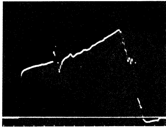
Fig. 7 - An overall record of an aluminum free surface exciting a magnetic probe. Time marks are spaced 100 nsec apart. Air shock causes the central portion of the record to be distorted. The peak signal represents the time for the aluminum to cross a 3-mm gap. For the geometry employed the initial sensitivity coefficient is about 3-V/mm/ \mu sec.
