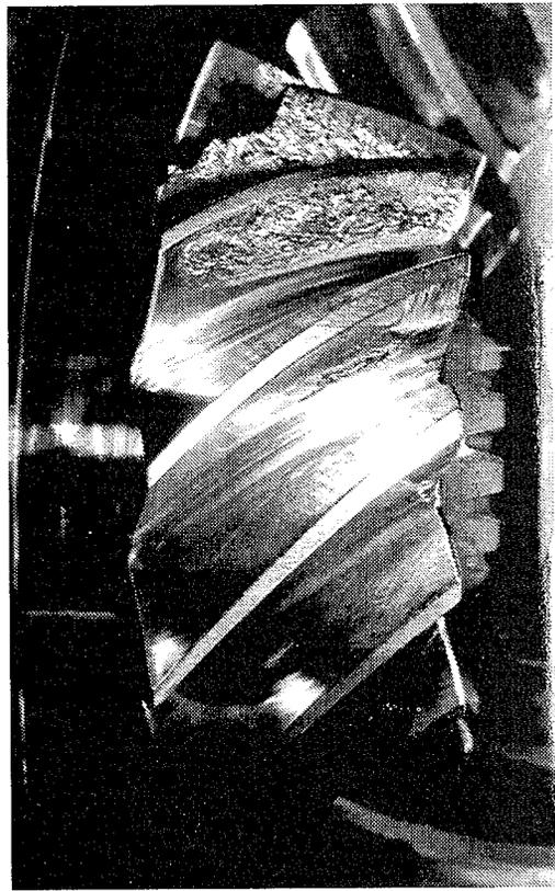
Figure 8.—Pinion damage at  $t = 17.79$  hr (end).
