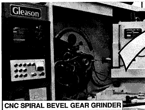
Figure 4.—Spiral bevel gear grinding.
