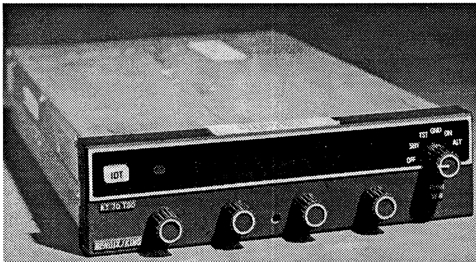
FIGURE 3. MODE-S TRANSPONDER. Mode-S transponders, similar to the panel-mount model pictured here, with a retail price of approximately $3000, can provide data link capability to General Aviation aircraft.
