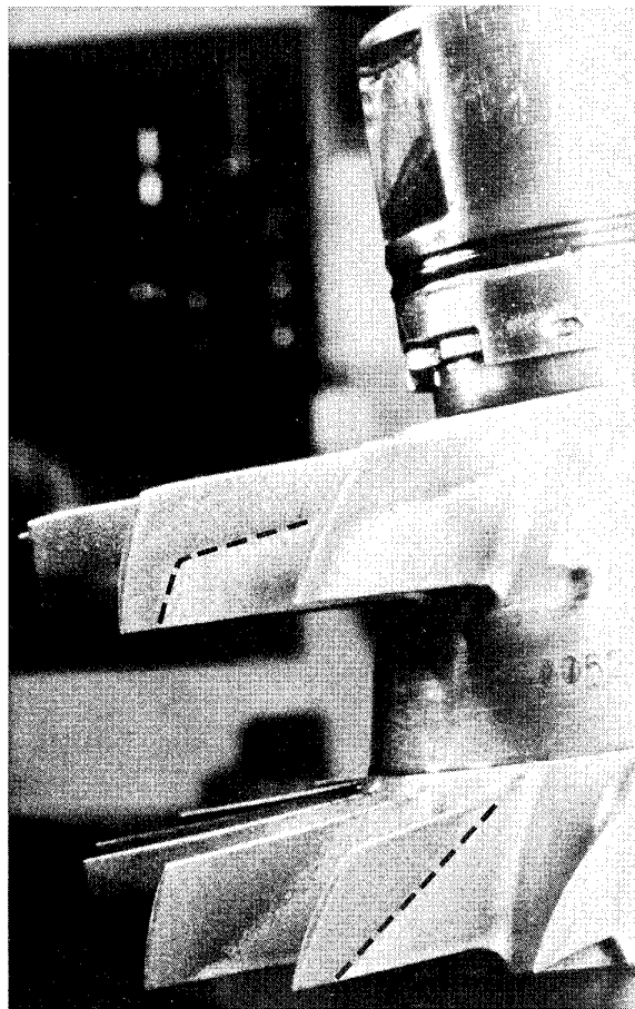
Fig. 9 The same blades as shown in figures 1c and 3 after 200 h service with an aluminium pigmented coating
