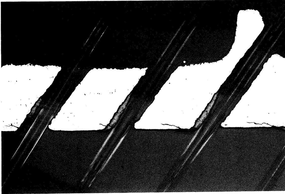
Fig. 12 Longitudinal section through cracked cooling channels showing nickel containing deposit in the channels. Deposit thickness approx. 80 \mu\text{m} , channel width at this position approx. 260 \mu\text{m} .
