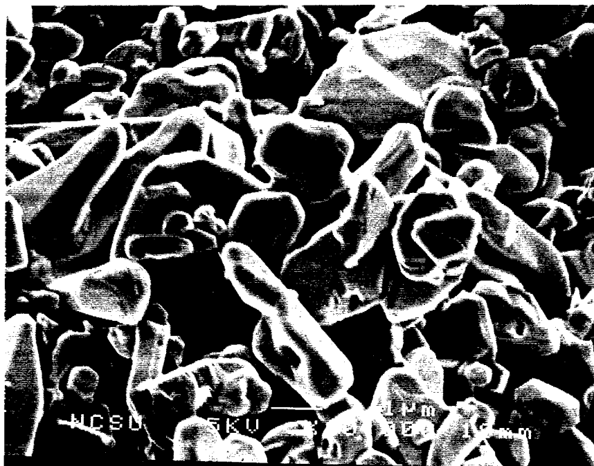
Figure 4. SEM image of the powder obtained using the Ga + NH 3 process route.
