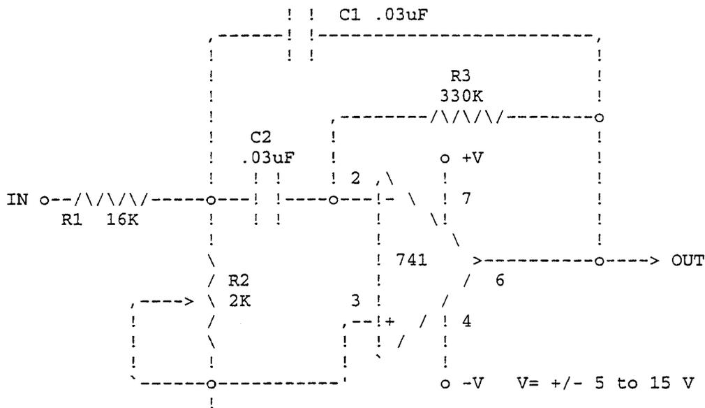
Audio Filter for SARA Telemetry Decoding.
