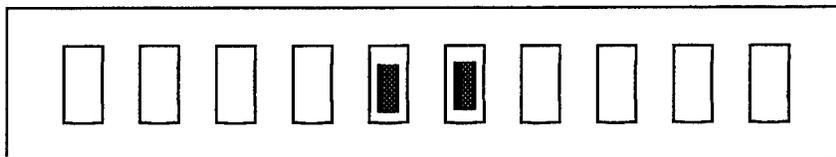
If the tuning indicator looks like the one below, the frequency from your speaker is too low to copy the signal. Slowly tune the VFO and make the frequency higher.
