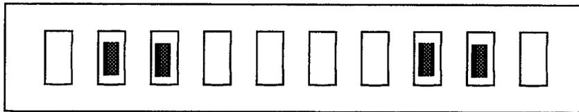
If the tuning indicator looks like the one below, adjust the frequency of your transceiver to achieve tuned-in display.
