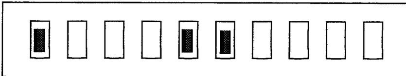
If the tuning indicator looks like the one below, adjust the frequency of your transceiver to achieve the tuned-in display.
