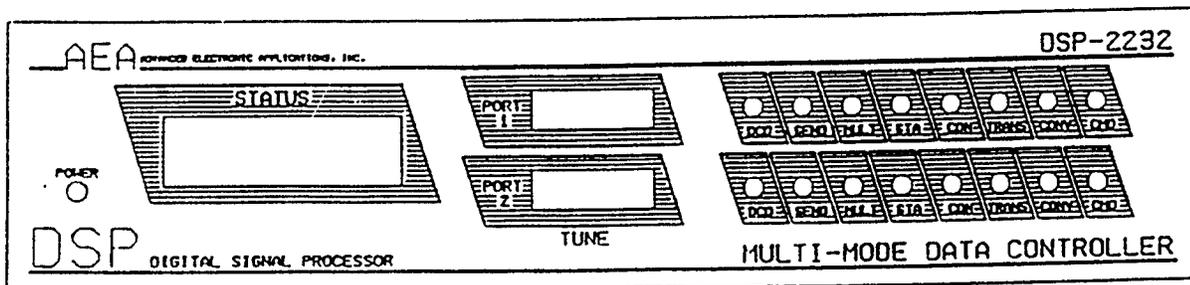
Fig.2.2.DSP-2232 Front Panel Controls and Indicators
