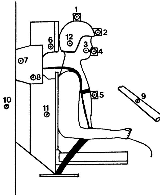
\* Fiducial target locations 6, 8 and 11 vary with respect to seat back angles. Below are x, y and z dimensions for seat back angles of +5, -5 and -10 degrees.
