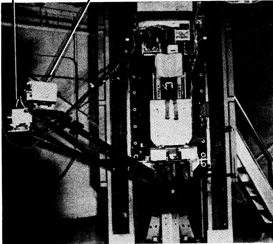
FIGURE A-9: ONBOARD CAMERA LOCATIONS
