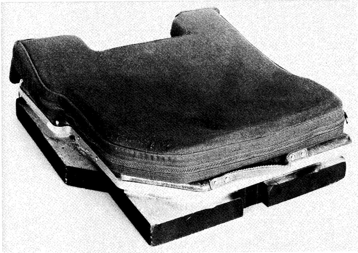
FIGURE 1. OPERATIONAL F-4 EJECTION SEAT CUSHION
