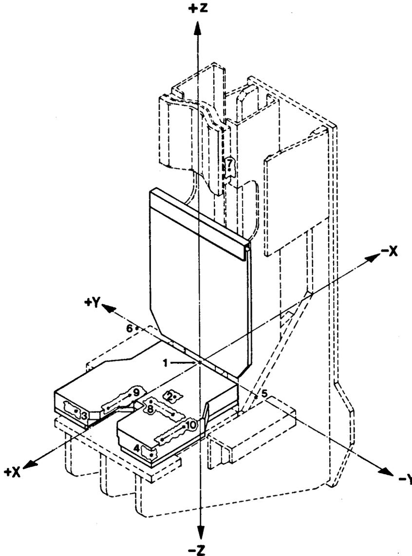
FIGURE A-4: LOAD TRANSDUCER LOCATIONS
