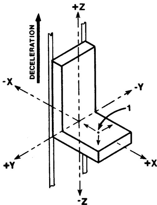
1. Typical fixed load cell and load link mounting point. Direction of arrows indicate direction of force applied to produce a positive output.
