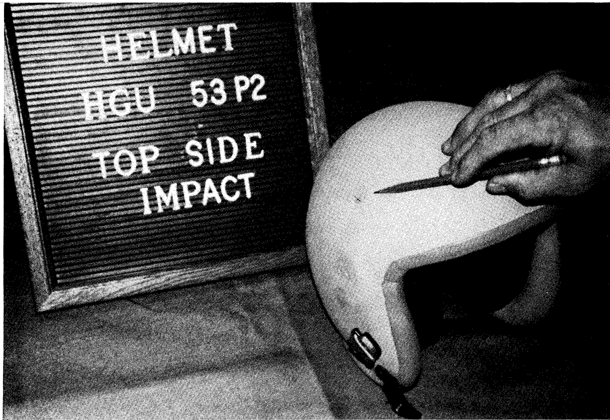
FIGURE 27. POINT OF IMPACT FOR 50 FT-LB IMPACT ENERGY TEST
