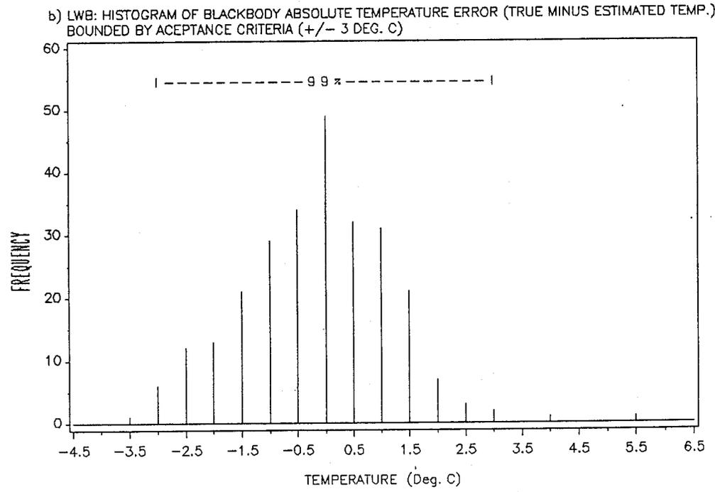
Figure 6. Blackbody calibration analysis for LWB data, no calibration correction needed
