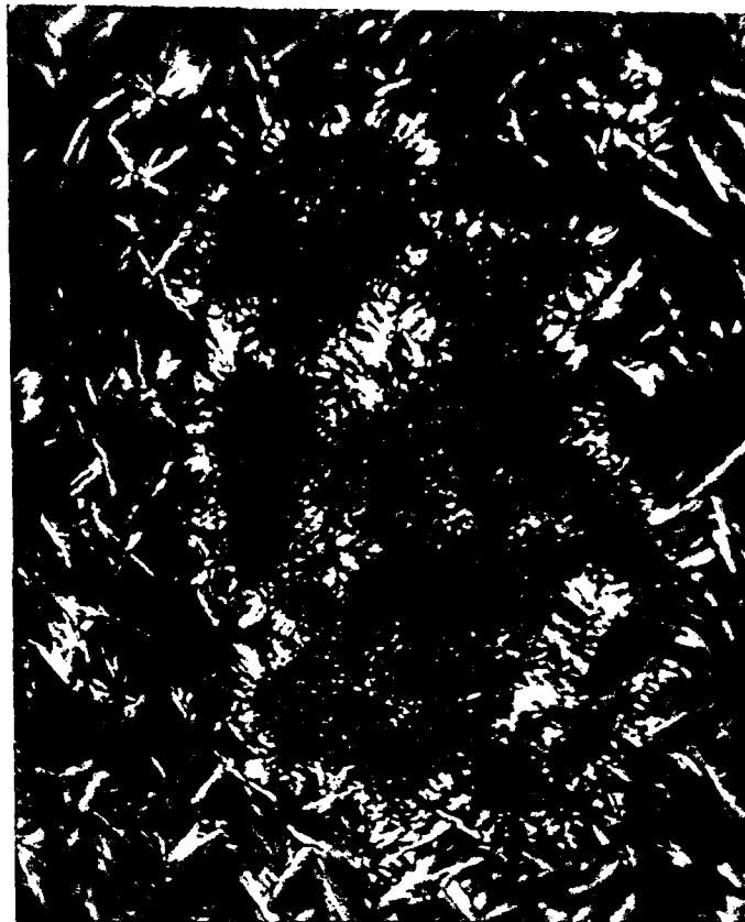
Figure 29. Ganex WP-660/Nitroethane Droplets in Polywax 600/Nitroethane Gel (400X).
