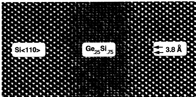
Fig. 5(a). Lattice image of Si/Ge 0.25 Si 0.75 /Si quantum well structure, viewed in <110> cross-section.
