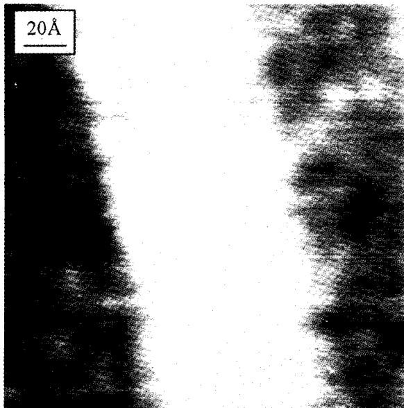
Figure 2. Annular Dark Field image of an 80 Å wide GaAs/In 0.2 Ga 0.8 As/GaAs quantum well. The two pictures display the same digitally recorded data set. The (110) atomic columns are seen in the GaAs in the upper image and in the In 0.2 Ga 0.8 As quantum well in the lower image. The atomic structure is continuous through the quantum well (specimen courtesy of Y. Chen).
