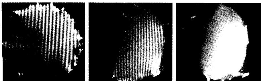
a b c Figure 3 Disappearance of the interference fringes as the beams are separated by reducing the biprism potential. See text.
